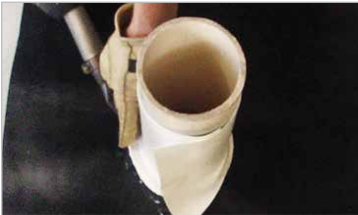
STEP 4. Final weld NR to target piece
