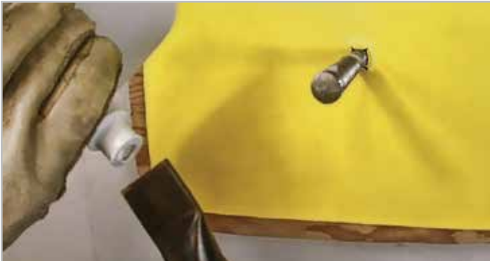
STEP 4A. Heat trimmed PF-150 cut end
