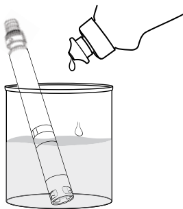
Figure 73 Cleaning the pH and pH/ORP sensor with dish soap
