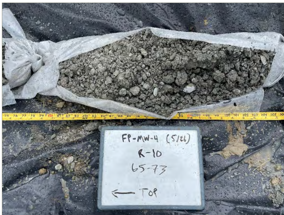
Exhibit D-4: Photo of PVC Core Bag from Sonic Drilling at Exploration FP-MW4
