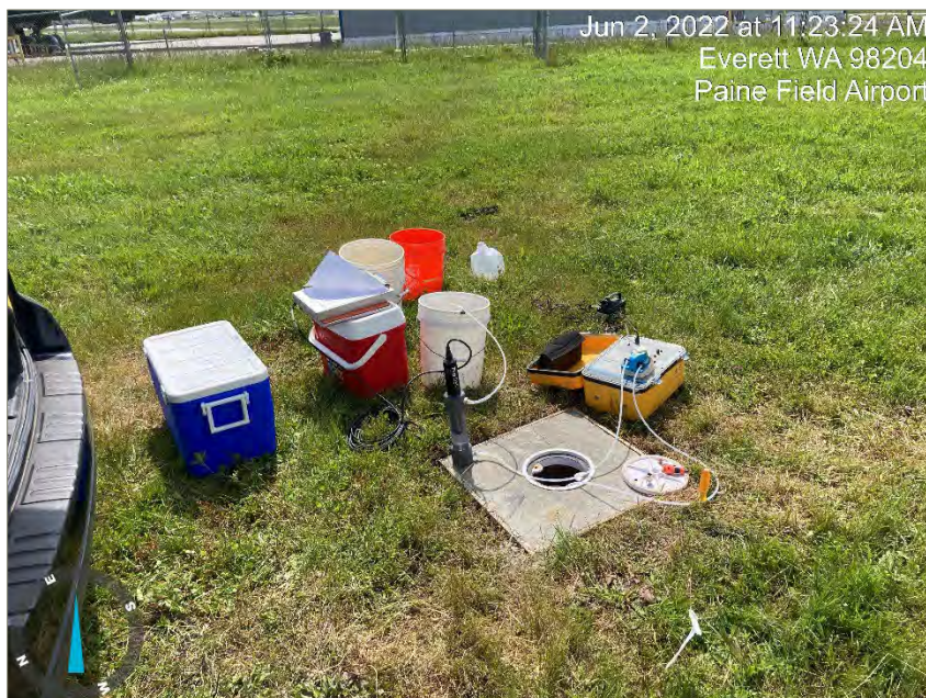
Exhibit D-9: Photo of a Typical Setup of Groundwater Purging Equipment Using a Peristaltic Pump
