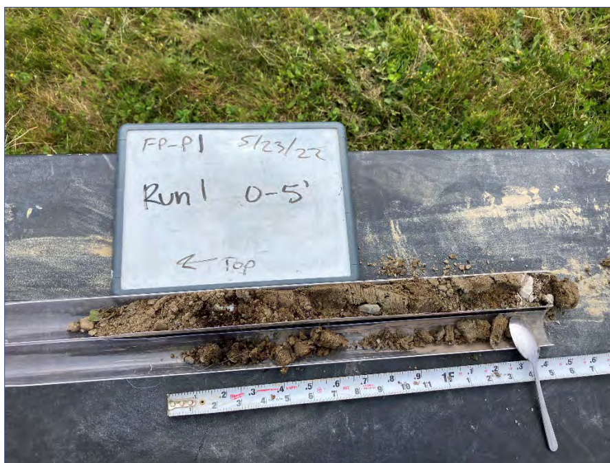
Exhibit D-2: Photo of Sliced PVC Liner and Soil Core at Exploration FP-P1
