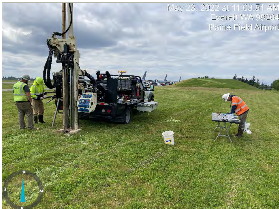
Exhibit D-1: Photo of Direct-Push Drill Rig at Exploration FP-P1 (View Direction is South)
