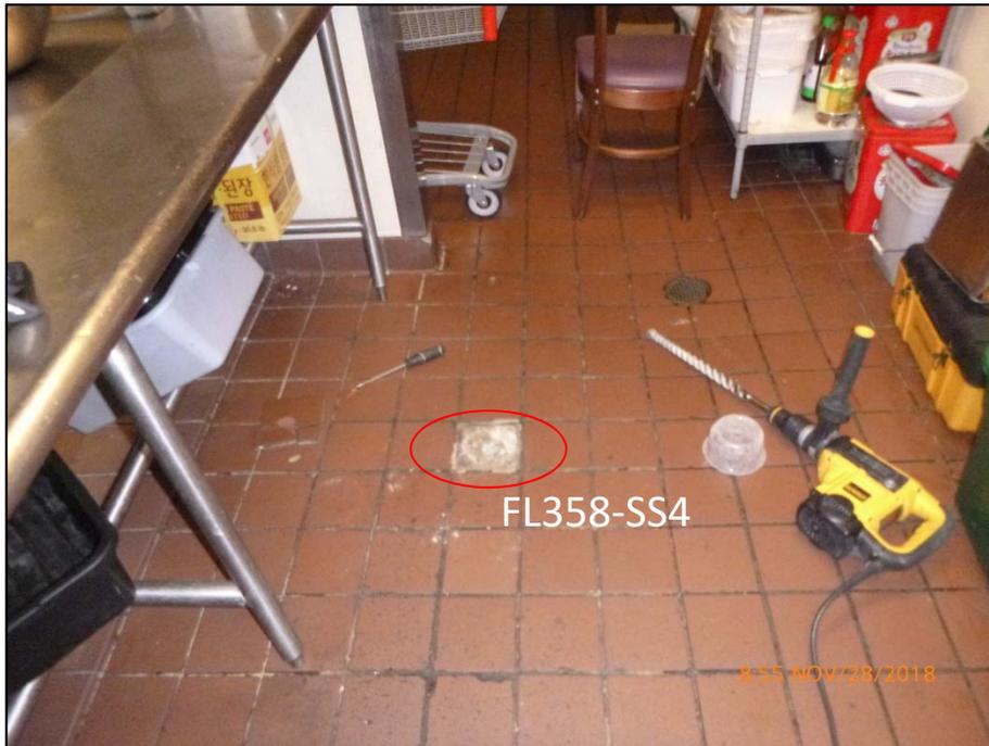
Photograph 1 – Passive sub-slab soil vapor sample location SS4, installed in kitchen of the Western Garden restaurant. Masonry drill and shroud at right of sample location.
