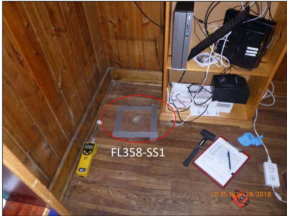
Photograph 3 – Completed passive sub-slab soil vapor sampler installation at location SS1 at the cashier station in the Western Garden restaurant. Field instrument (PID) visible surrounding location.
