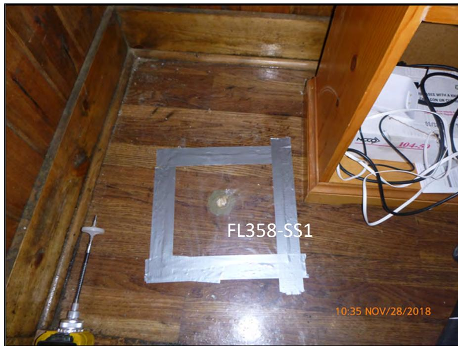
Photograph 4 –Detail of sample location SS1 showing cork in center of slab penetration, surrounded by bentonite seal and waterproof plastic sheet and tape.
