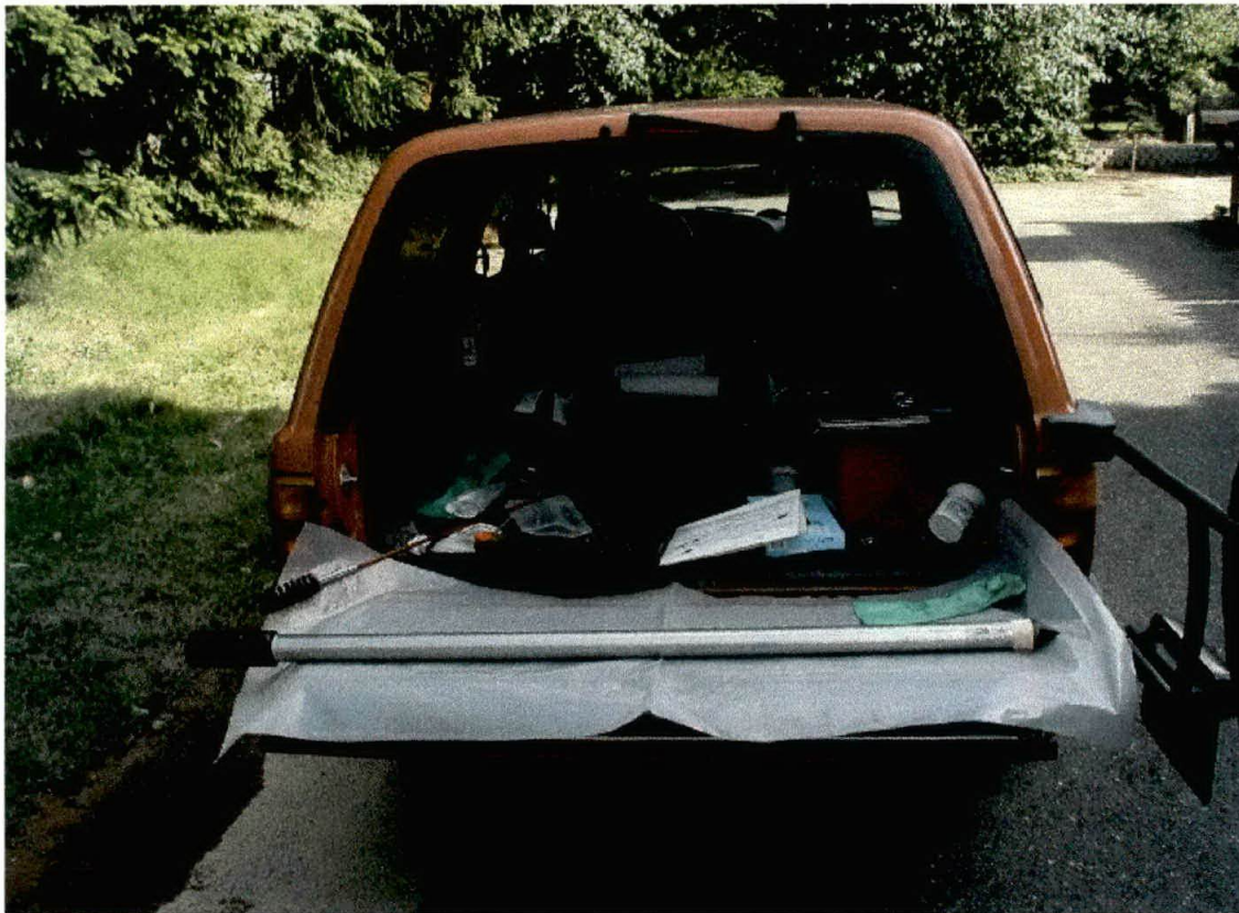
Photo 10. View of the Hydropunch sampler that was used during the drilling of the MW-13 boring to collect groundwater samples from the subsurface aquifer at depths of 120, 160 and 180 feet below ground surface.
