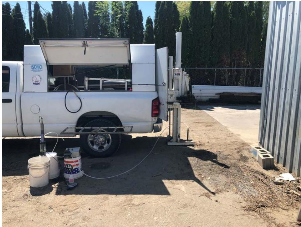
Temporary well point sampling from boring GEI014-DP2 (view looking south).
