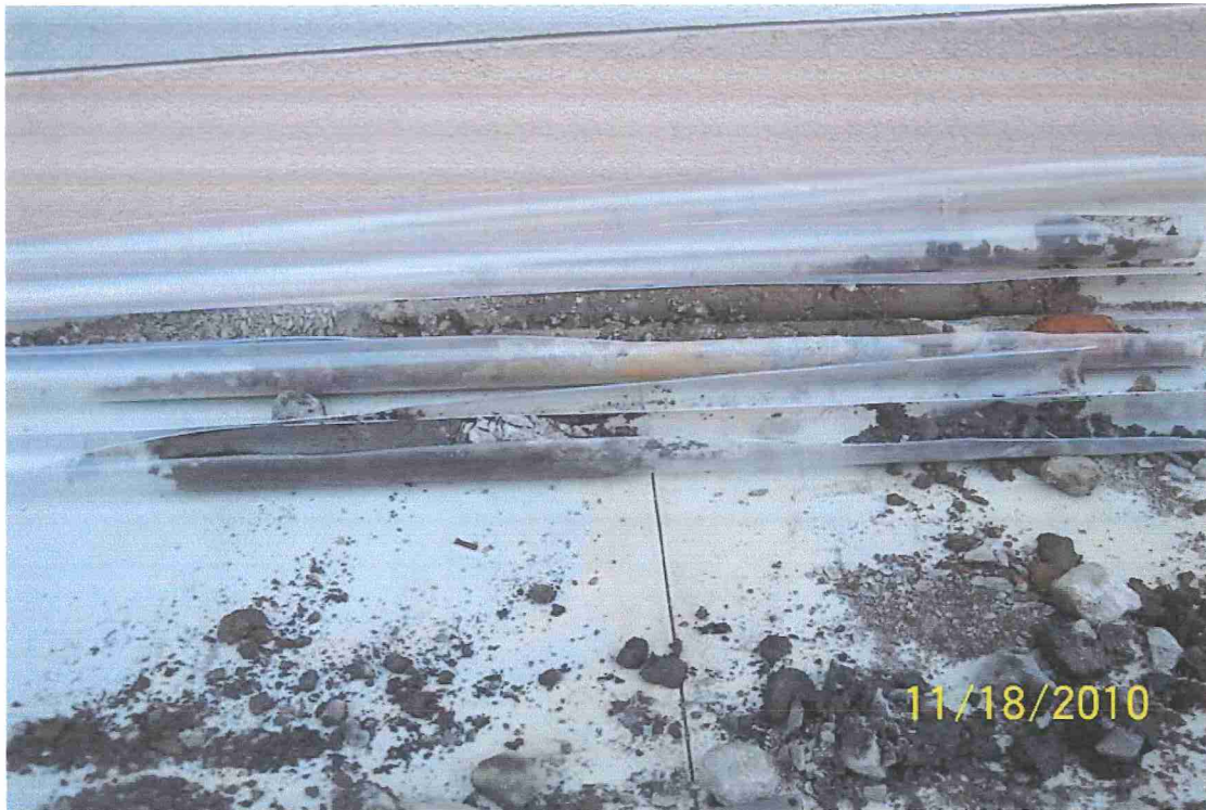
TYPICAL SOIL PROFILE TO 12 FEET BGS.
