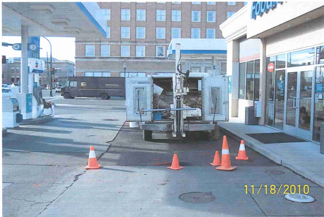
SAMPLING AT THE FORMER UST LOCATION.
