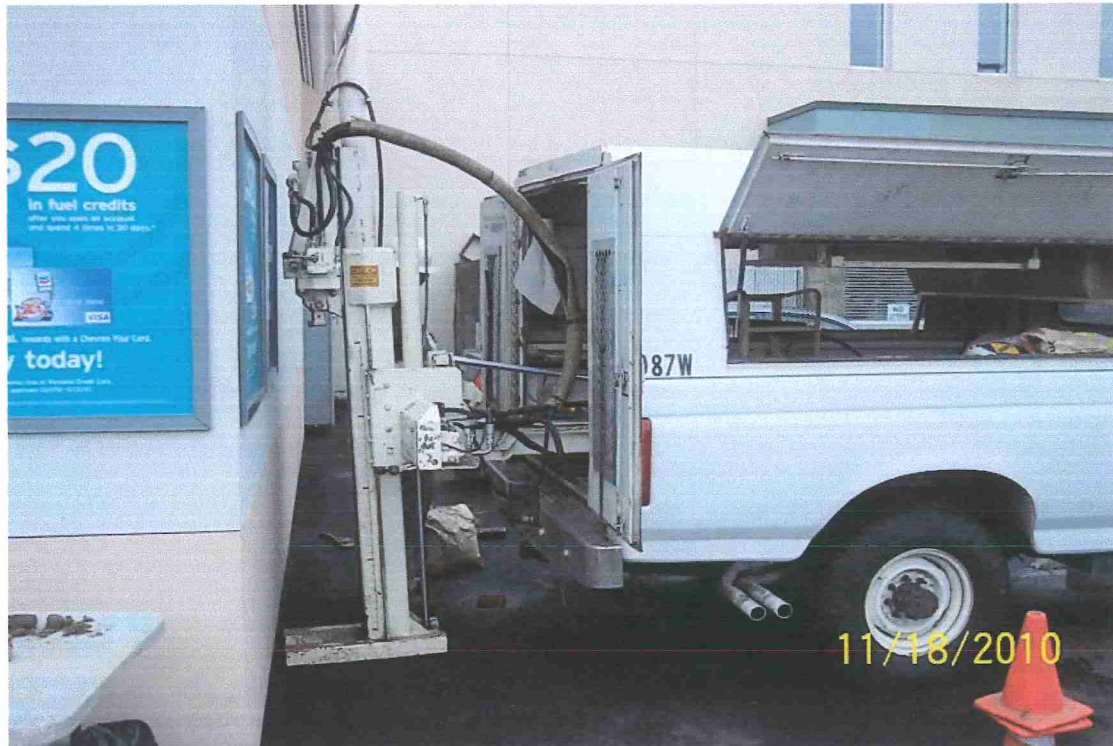
SAMPLING AT THE FORMER HYDRAULIC LIFT LOCATION.
