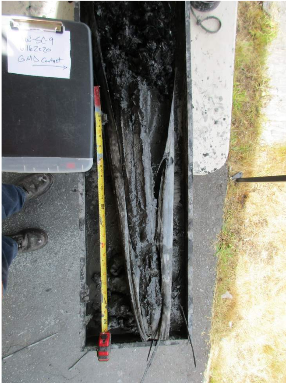
Photograph No. 11 – Lower section of sediment core IJW-SC-9, approximately 5.5 to 9.3 feet bml. View of GMD contact at approximately 6.2 feet bml. Photograph taken on 6/16/2020.
