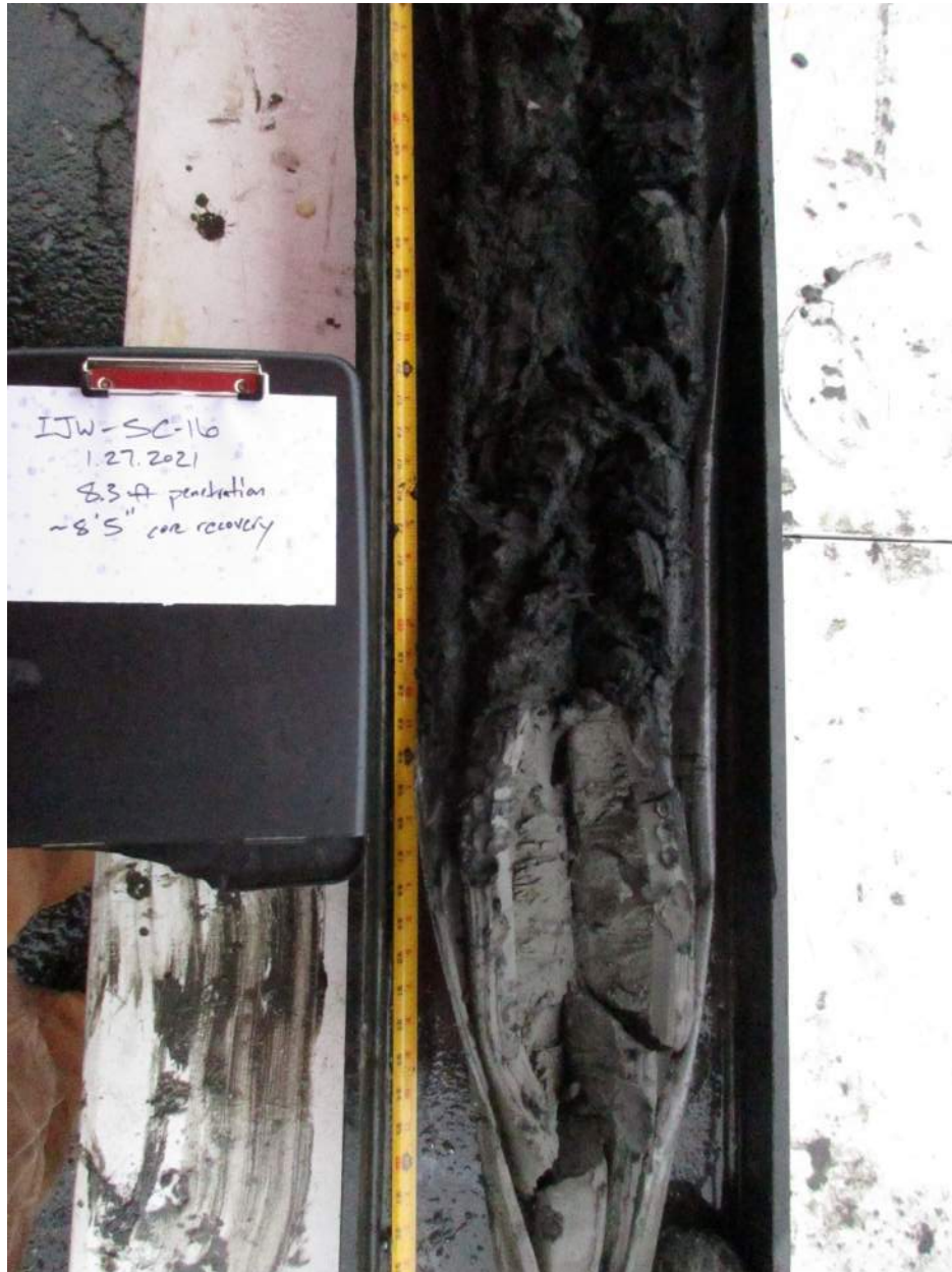
Photograph No. 21 – Sediment core IJW-SC-16, approximately 5.5 to 8 feet bml. View of GMD contact at approximately 7 feet bml. Photograph taken on 1/27/2021.
