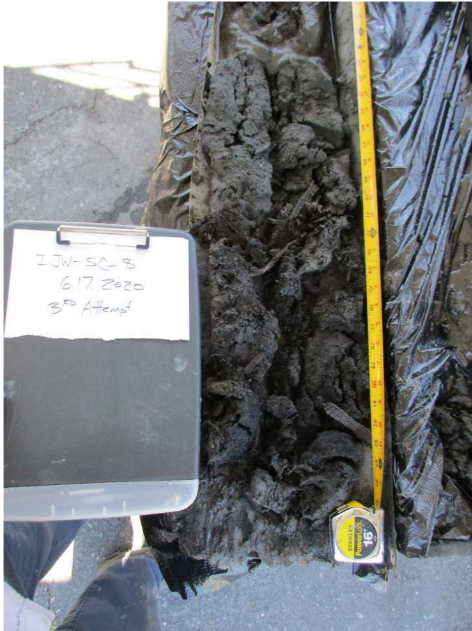
Photograph No. 9 – Lower section of sediment core IJW-SC-8, approximately 5 to 8.8 feet bml. GMD tagged at 8.8 feet bml. Photograph taken on 6/17/2020.
