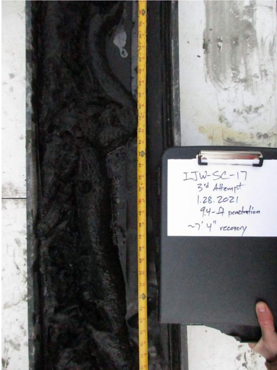
Photograph No. 22 – Sediment core IJW-SC-17 sediment material, approximately 3.5 to 5.5 feet bml. No GMD encountered. Photograph taken on 1/28/2021.
