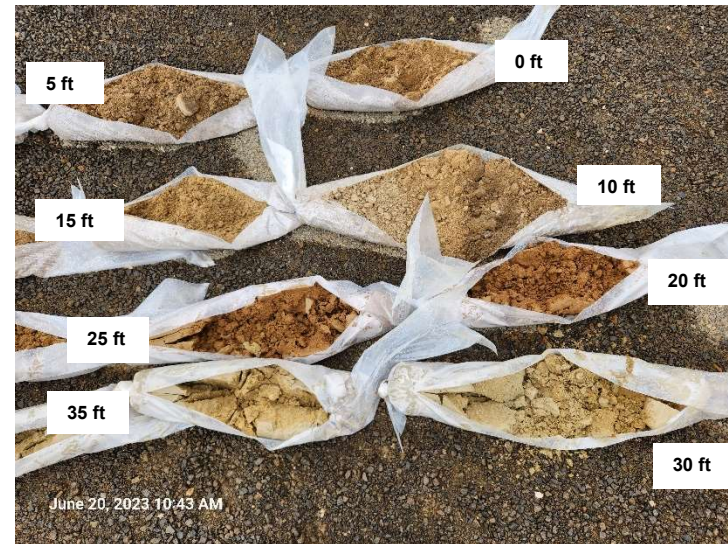
Photo 28. MW-5DR soil cuttings
