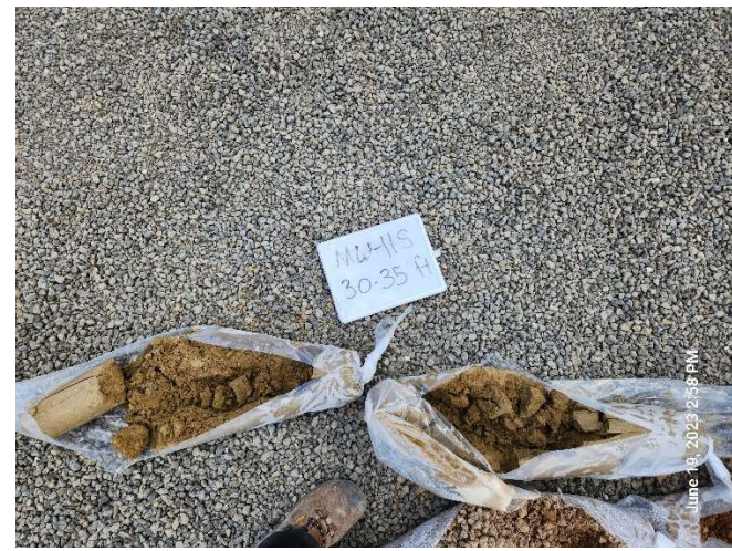
Photo 8. MW-11S soil cuttings; 30 to 35 feet
