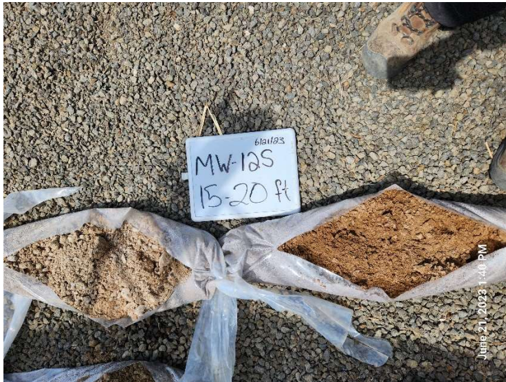
Photo 15. MW-12S soil cuttings; 15 to 20 feet.
