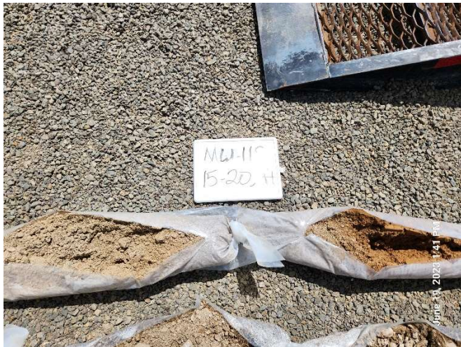
Photo 5. MW-11S soil cuttings; 15 to 20 feet
