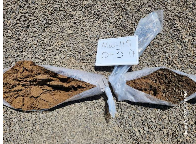
Photo 2. MW-11S soil cuttings; 0 to 5 feet
