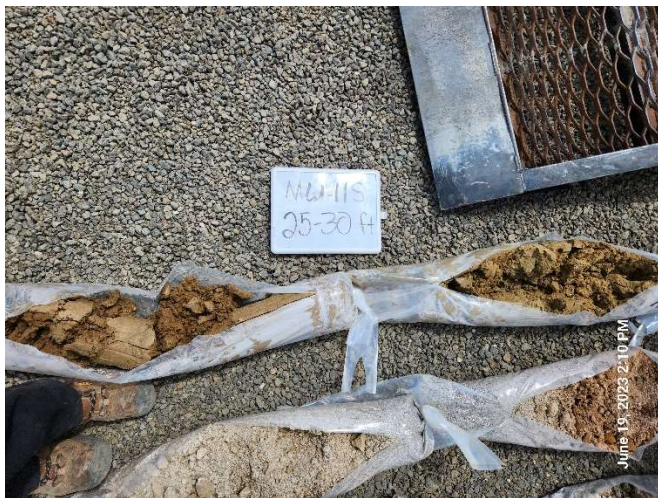
Photo 7. MW-11S soil cuttings; 25 to 30 feet
