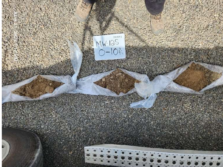
Photo 13. MW-12S soil cuttings; 0 to 10 feet
