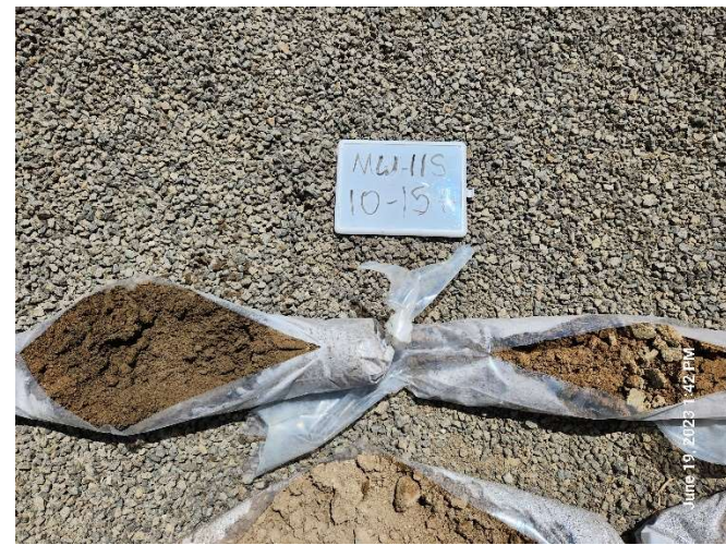
Photo 4. MW-11S soil cuttings; 10 to 15 feet
