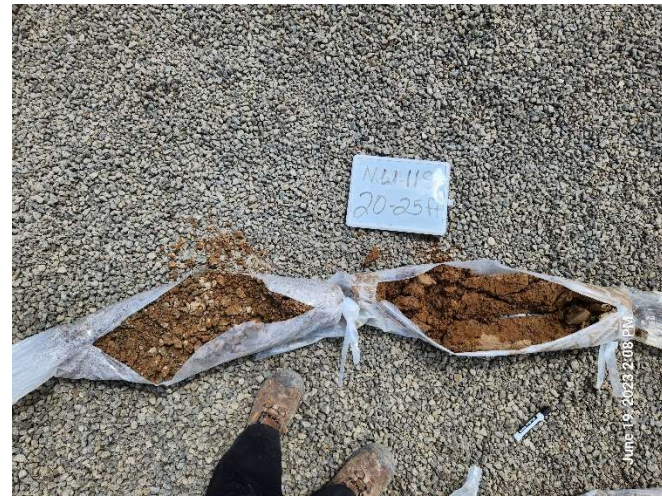
Photo 6. MW-11S soil cuttings; 20 to 25 feet
