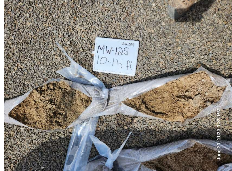
Photo 14. MW-12S soil cuttings; 10 to 15 feet
