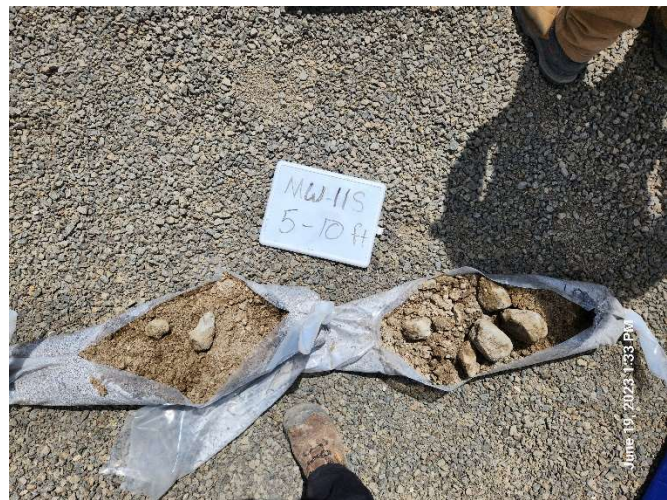
Photo 3. MW-11S soil cuttings; 5 to 10 feet
