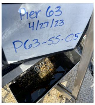
Photograph D-10 Homogenized Sediment Grab P63-SS-05
