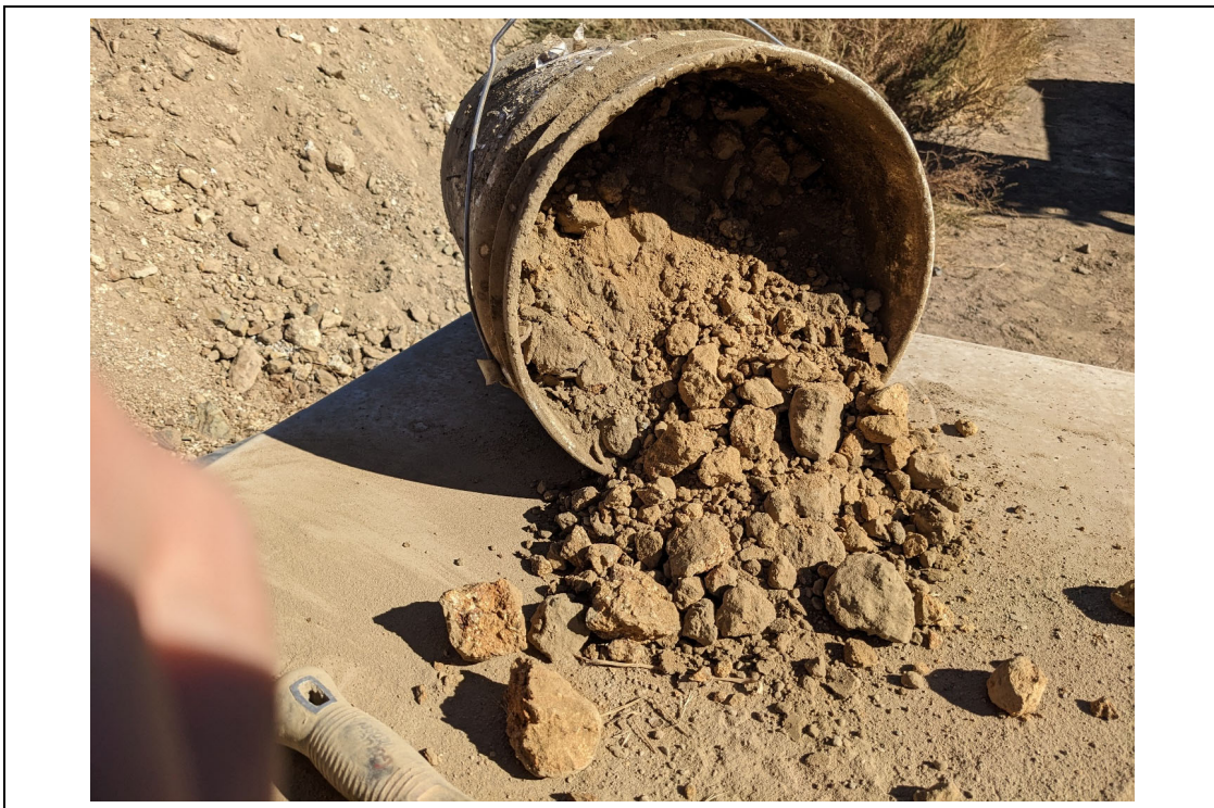
Weather basalt encountered at site T2.
