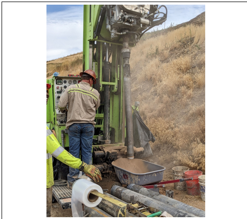
Example of a sample being released into a steel wheelbarrow.
