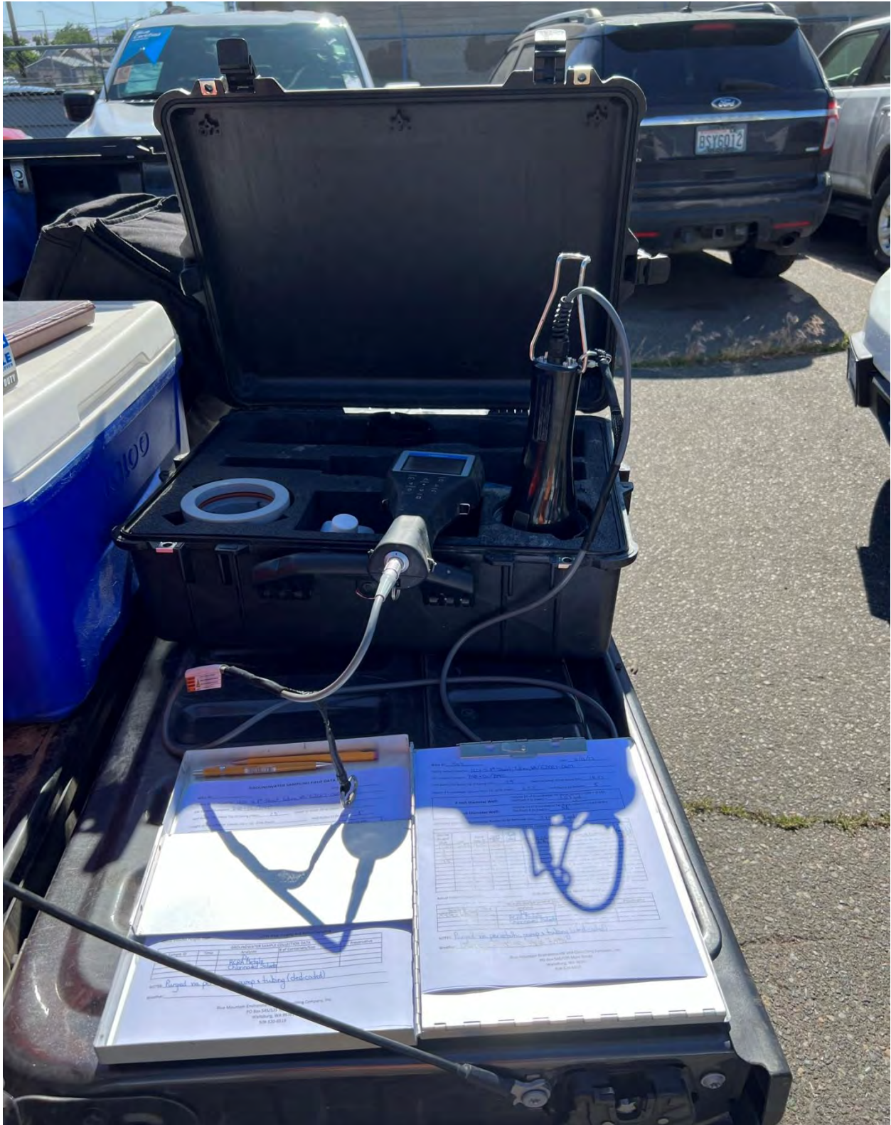
Photograph 11 – View of the Horiba U-52 used to assess groundwater parameters in the field on June 13, 2023.
