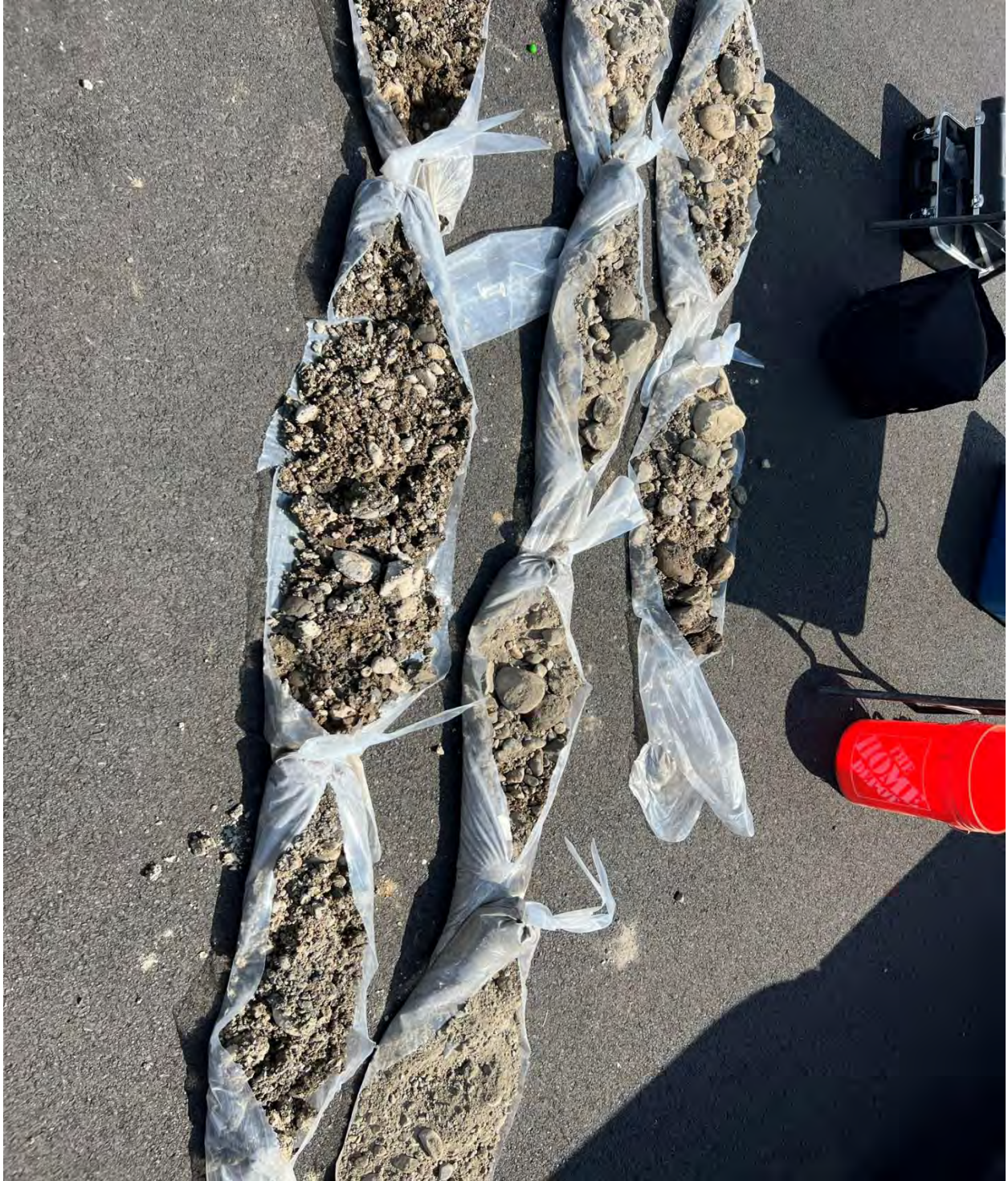
Photograph 4 – Soil cuttings from boring MW8 on May 19, 2023.
