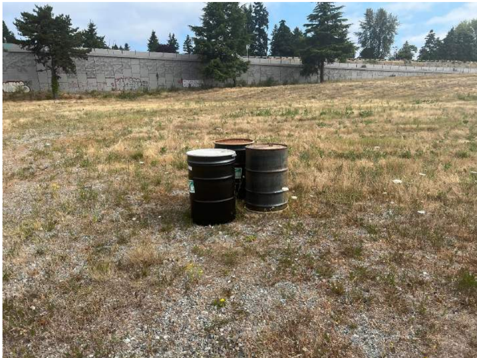
Photograph 6. Three purged groundwater drums ready for transport and disposal, photographed on July 12, 2023.
