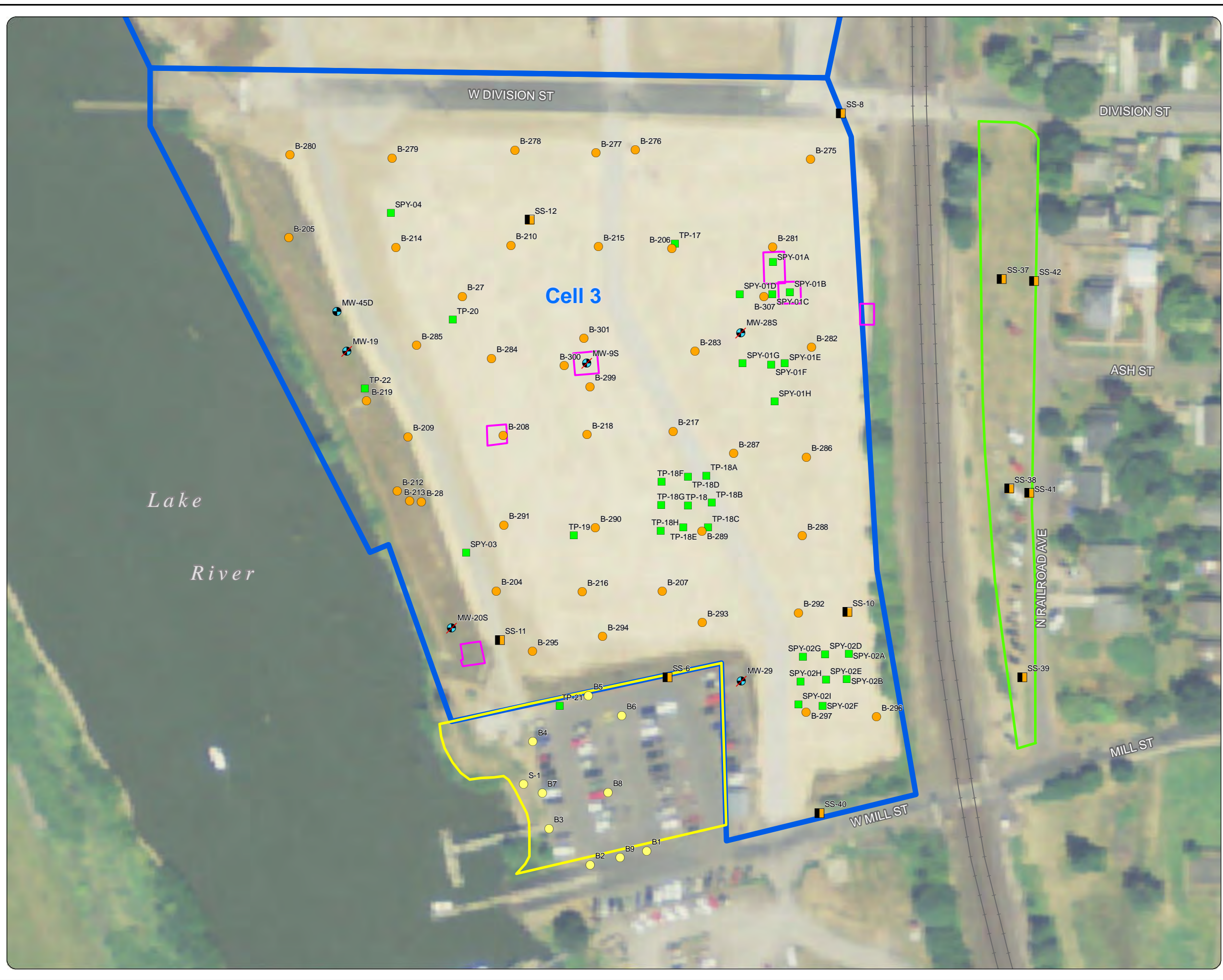
Figure 3-1 Cell 3, Port Marina, and Railroad Avenue Soil Sample Locations and Excavation Extents
