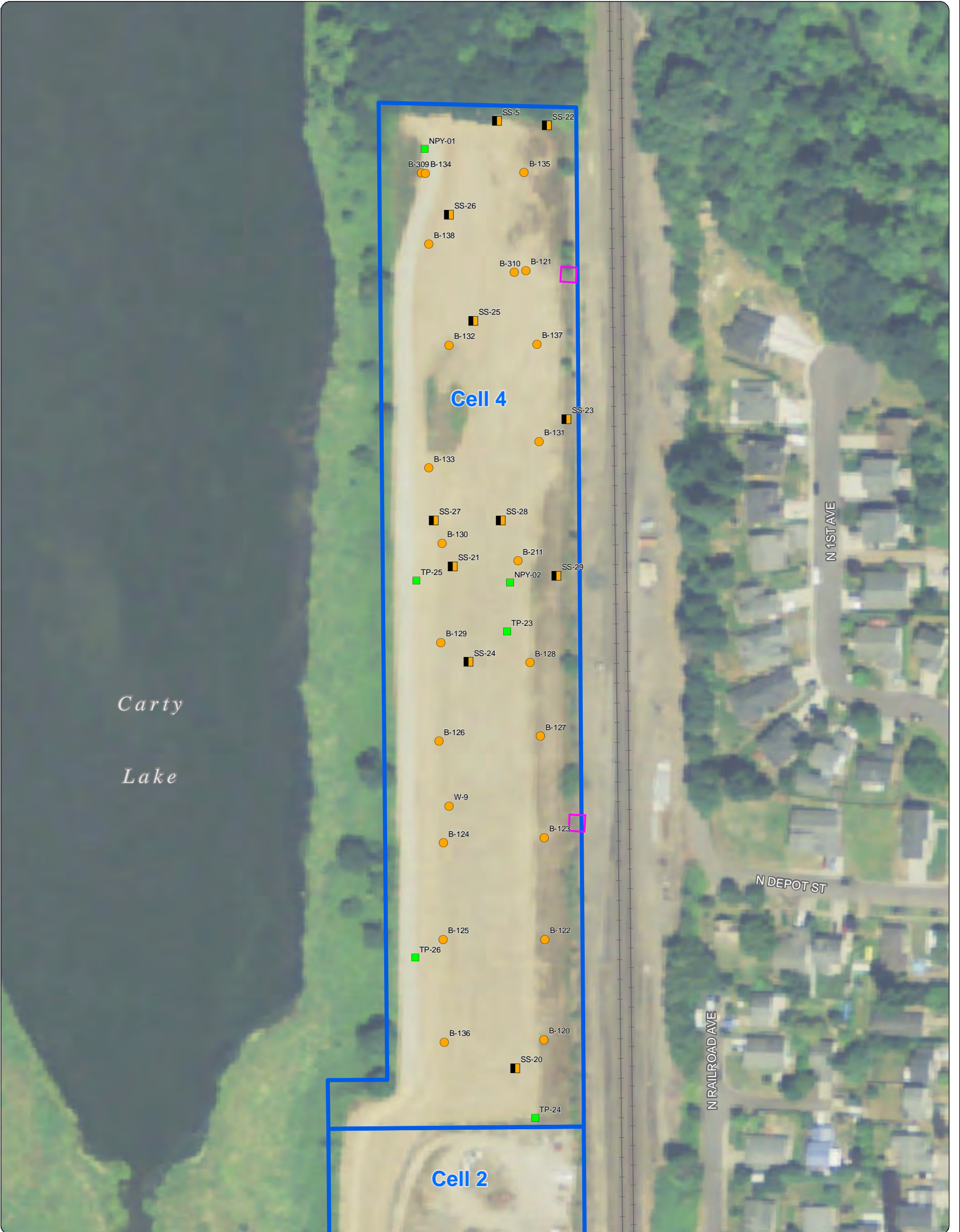
Figure 3-2 Cell 4 Soil Sample Locations and Excavation Extents Port of Ridgefield Ridgefield, Washington
