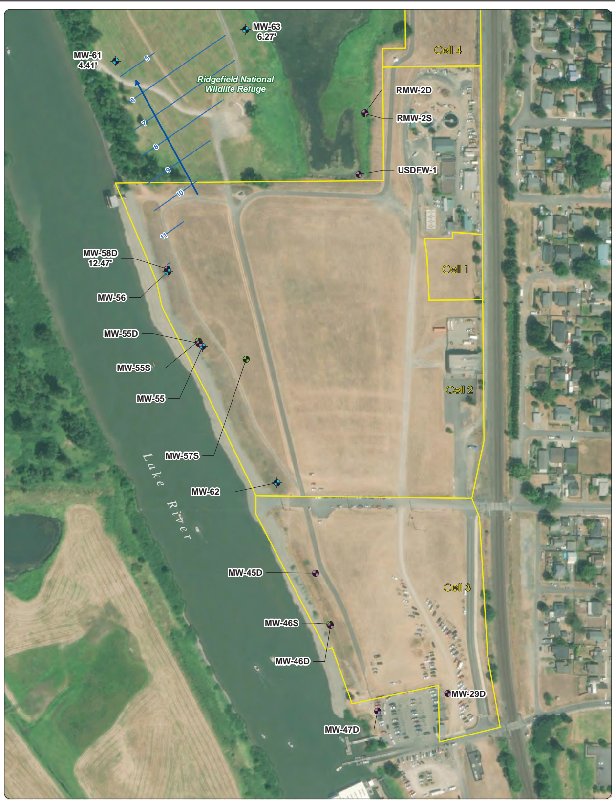
Figure 2 Groundwater Potentiometric Map for Lower Water-Bearing Zone
