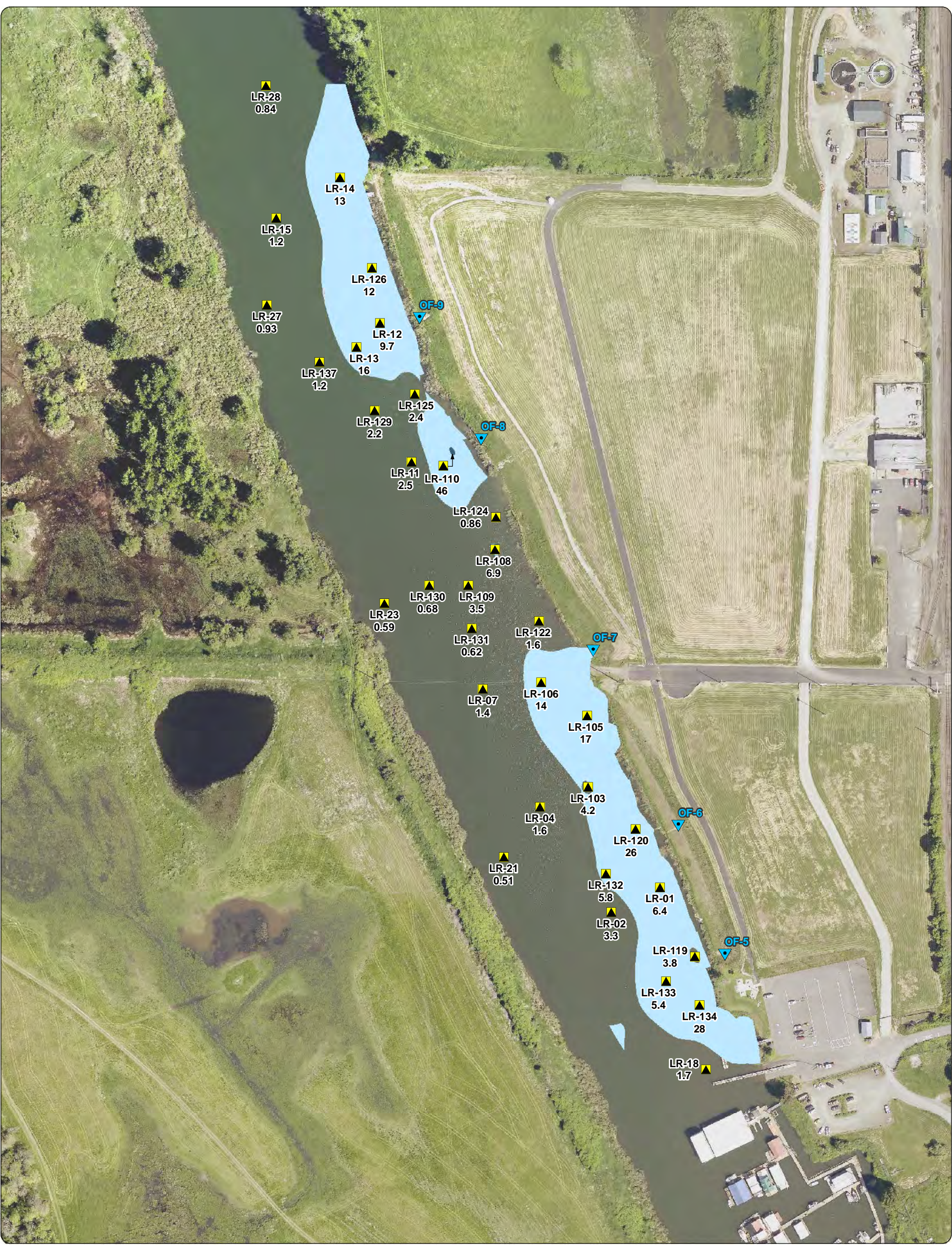
Figure 3 Predicted Post-Dredge Sediment Concentrations
