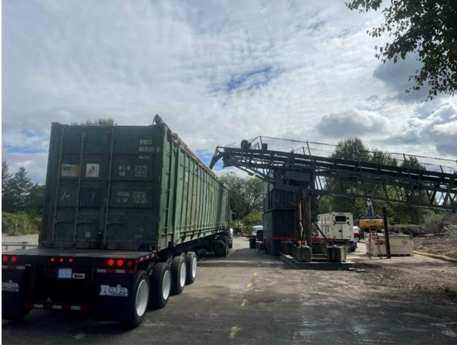
Photograph 5: Loading dross into haul bins (on truck trailer) using conveyor system.
