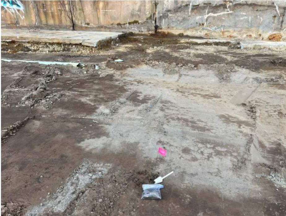
Photograph 17: Performance monitoring sampling activities (CS-25) using disposable scoop and ziplock bag for initial collection. View to the north. 10/23/2023
