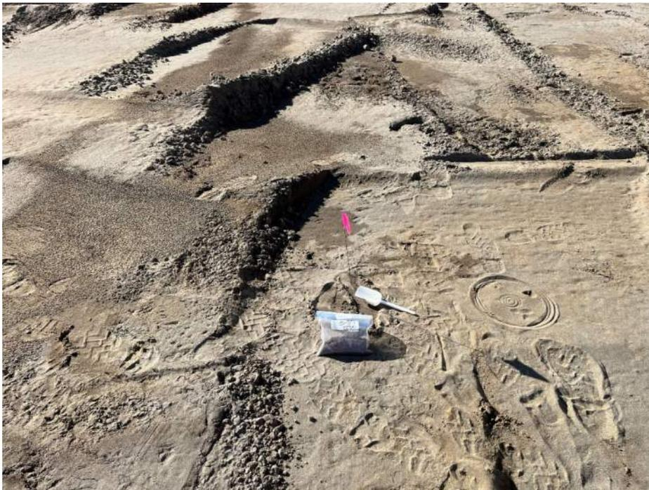
Photograph 20: Performance monitoring sampling activities (CS-35) using disposable scoop and ziplock bag for initial collection. View down. 10/30/2023
