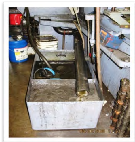
Photo 13-3: Circa 2008 photograph showing an example of the poor housekeeping practices with open containers and evidence of petroleum and solvent releases from the camshaft rinse areas.
