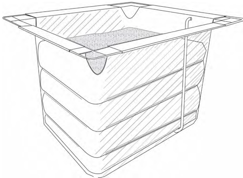
FIGURE 7 – FLEXBASIN™ CATCH BASIN INSERT SHOWN WITH FOUR PILLOWS
