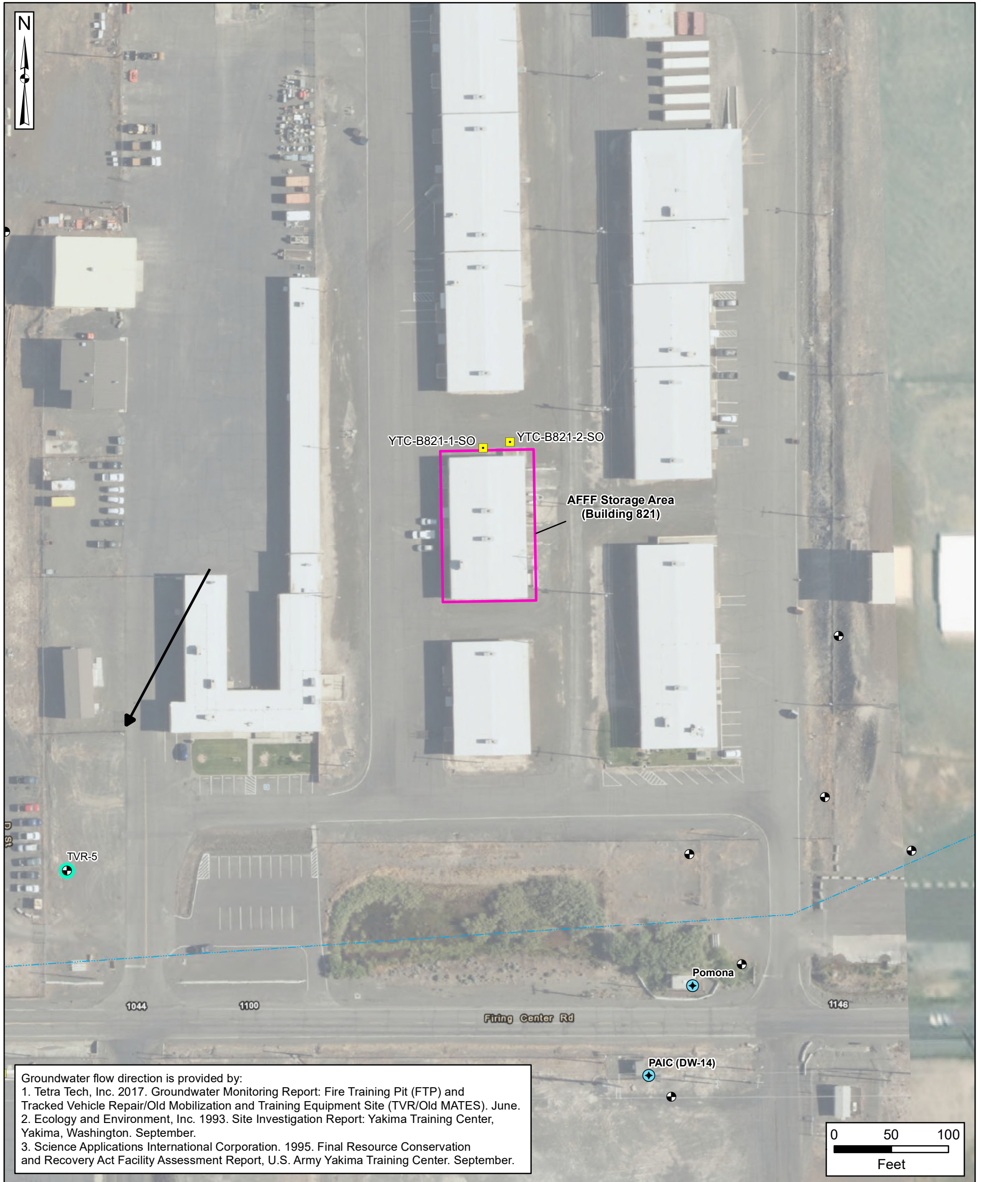
Figure 8 Proposed Sampling Locations - AFFF Storage Area (Building 821)
