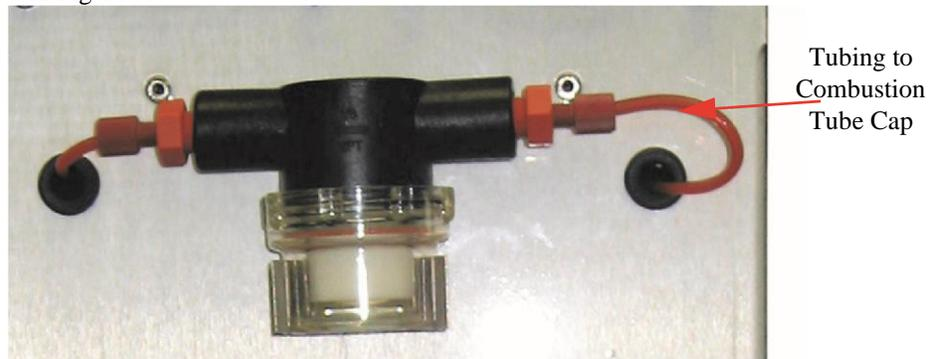
Figure 5.4. Tube Between Particulate Filter and Combustion Tube
