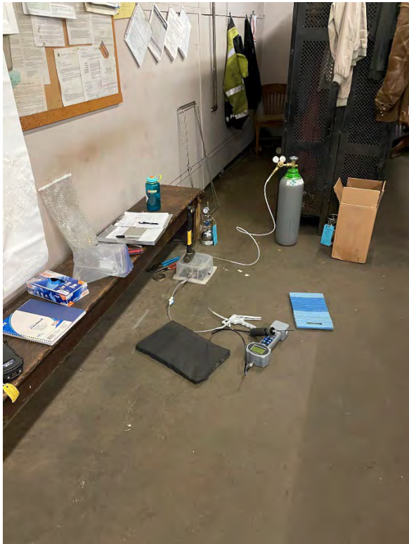
SBW SV-3 Sub-Slab Sample Location – Helium Shroud Setup
