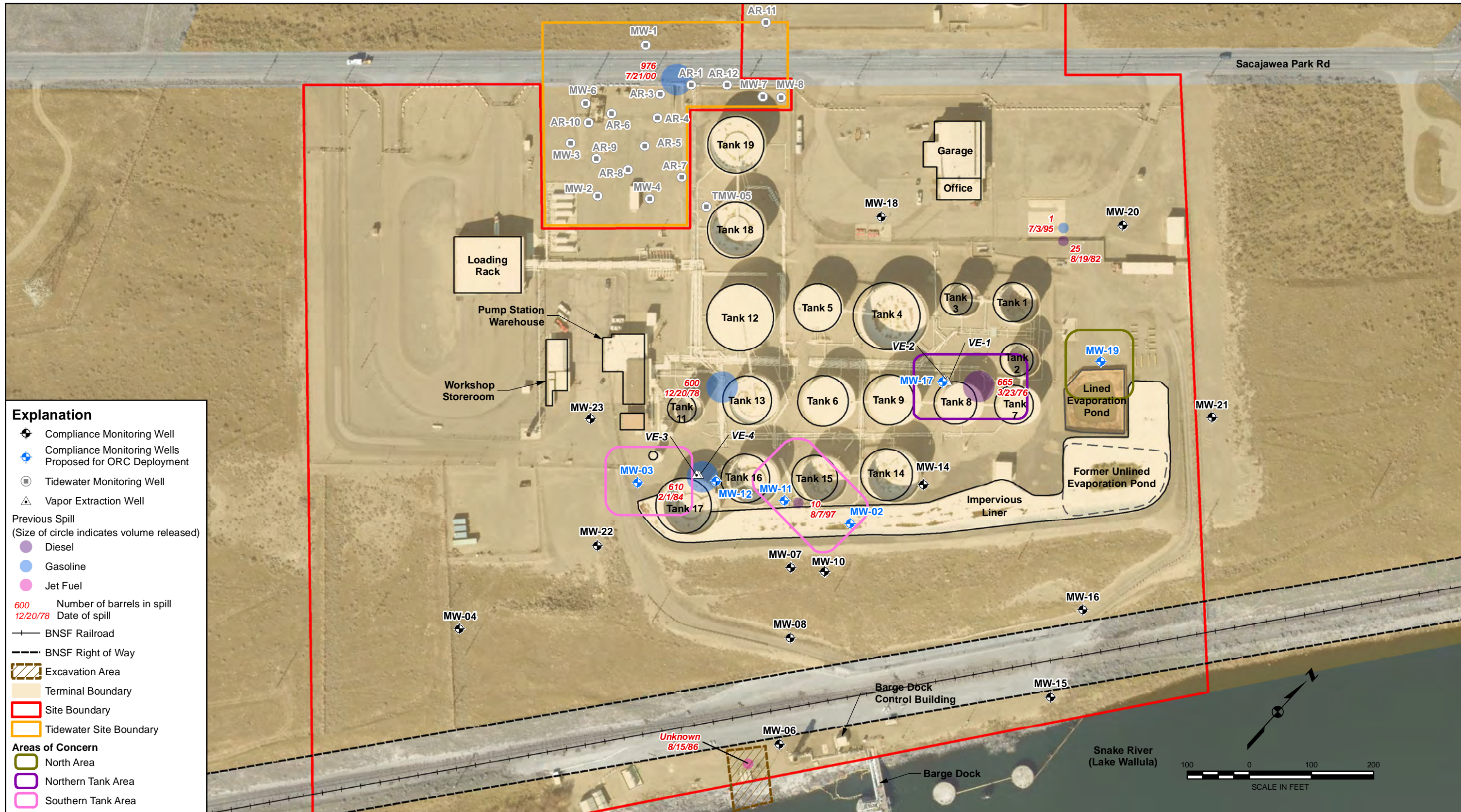
SITE MAP AND MONITORING WELLS PROPOSED FOR ORC DEPLOYMENT
