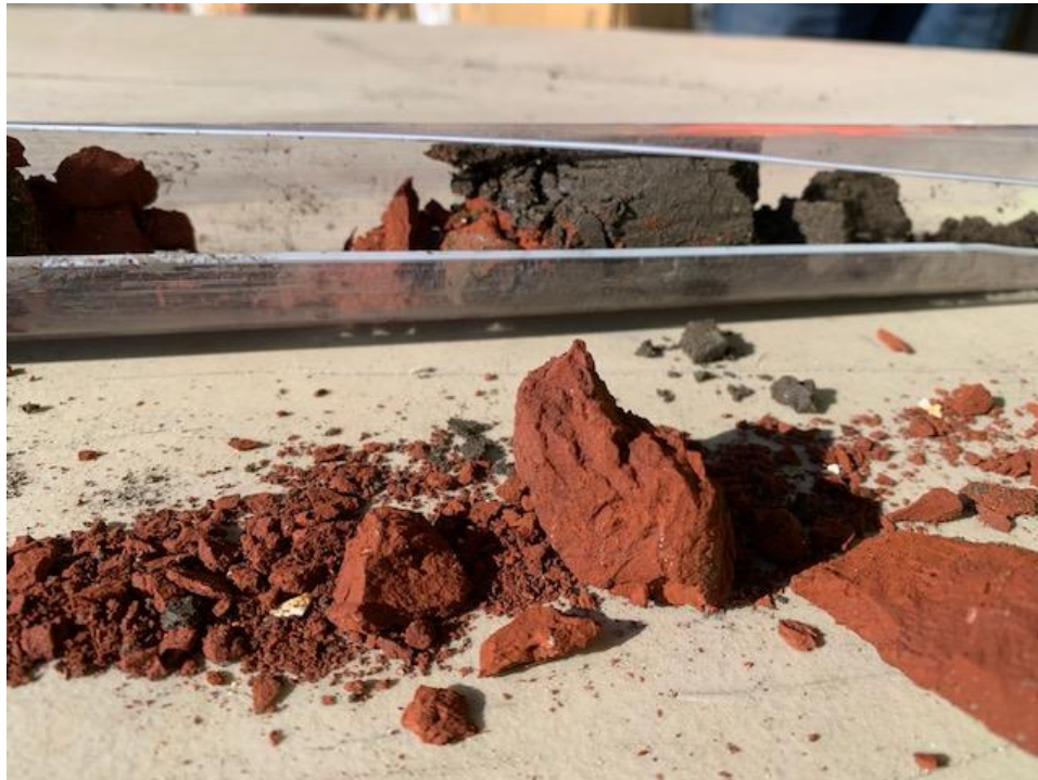
Photo 6: Red brick debris at the bottom of borehole B1 that lead to equipment refusal
