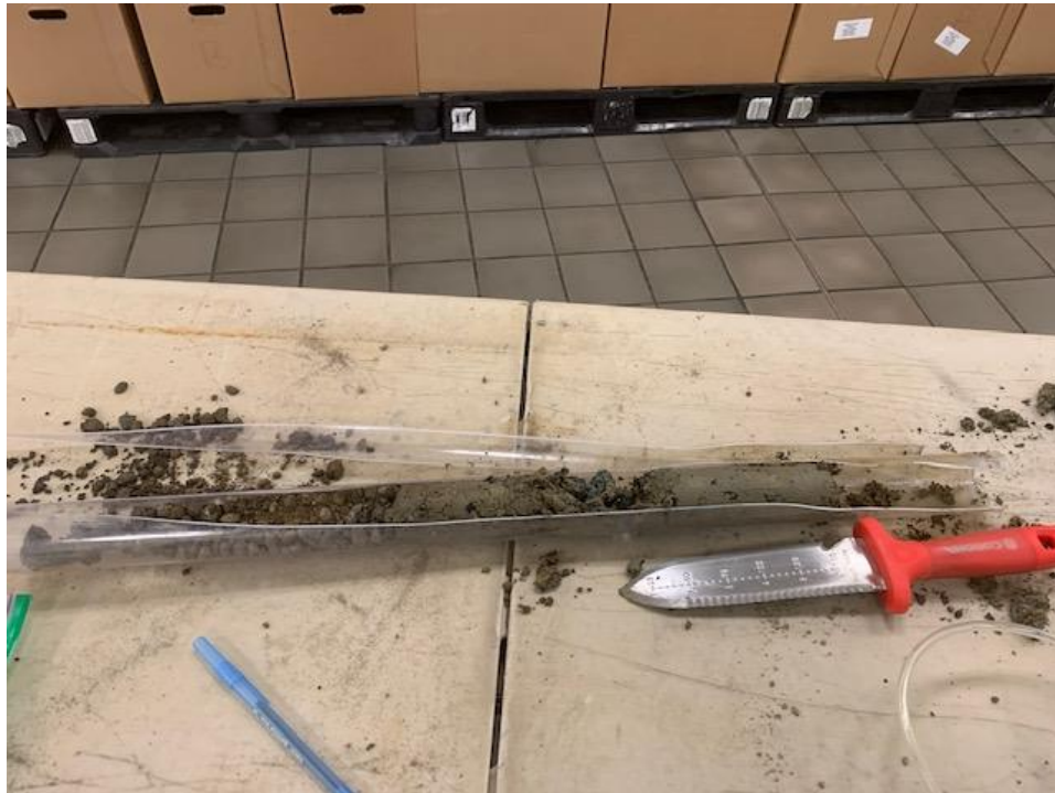
Photo 12: Boring B3; 6 to 9 foot depth
