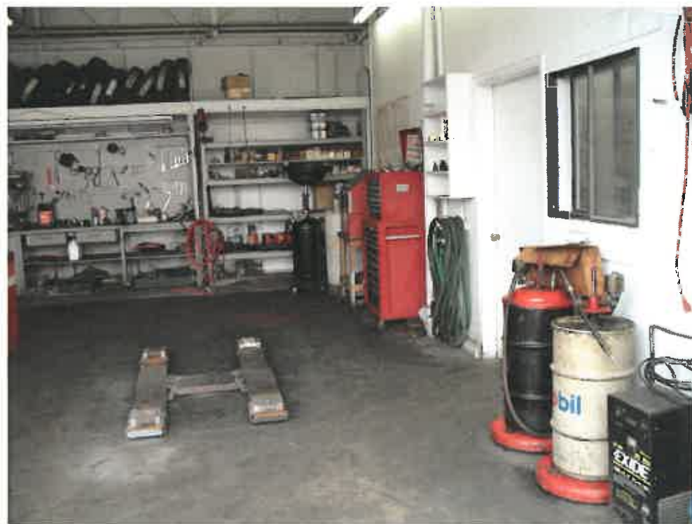
10. The eastern service bay, showing oil storage with secondary containment and a typical hydraulic, single-pole lift
