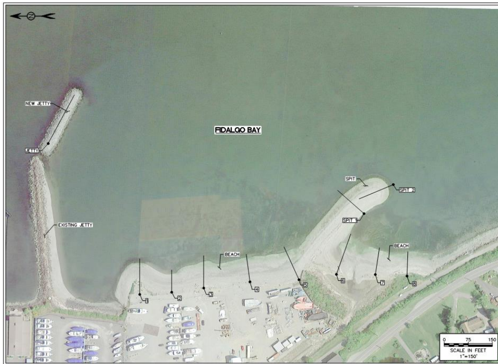
Figure 1. Plan view of project site showing transect locations along beach, spit, and new jetty extension structures
