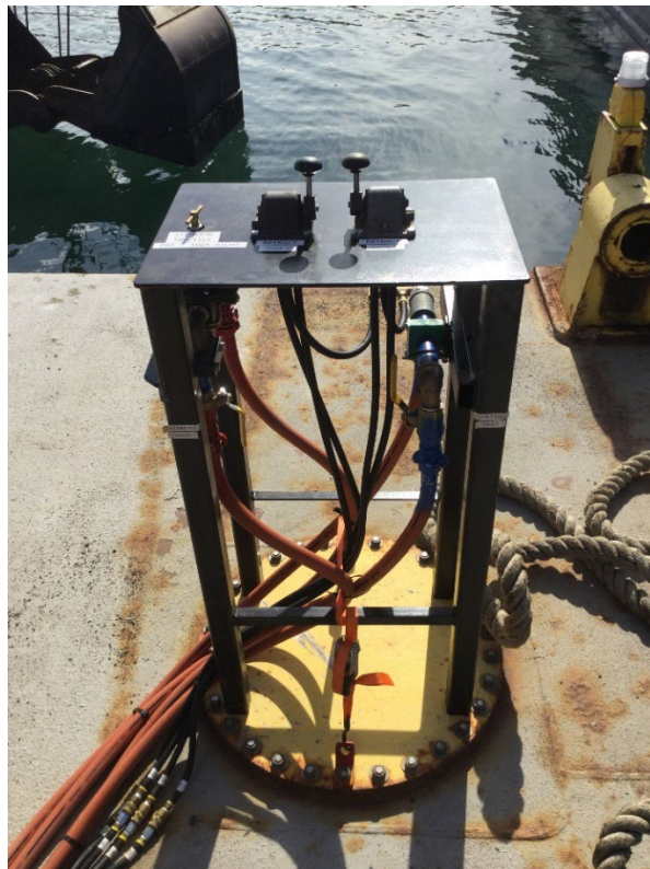
Photo #14: Pneumatic controls of 2-inch thin layer cap table.
