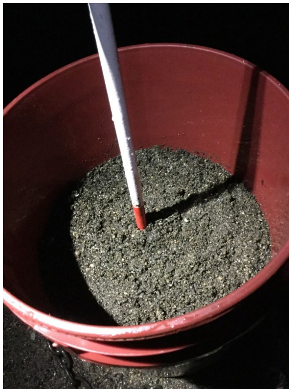
Photo #10: Rain bucket measurement collected using a painted metal rod. The rod was painted to specifically show the permissible range of thickness placed.
