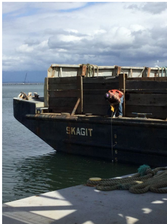
Photo 2: Measurement collected to approximate the draft of the barge
