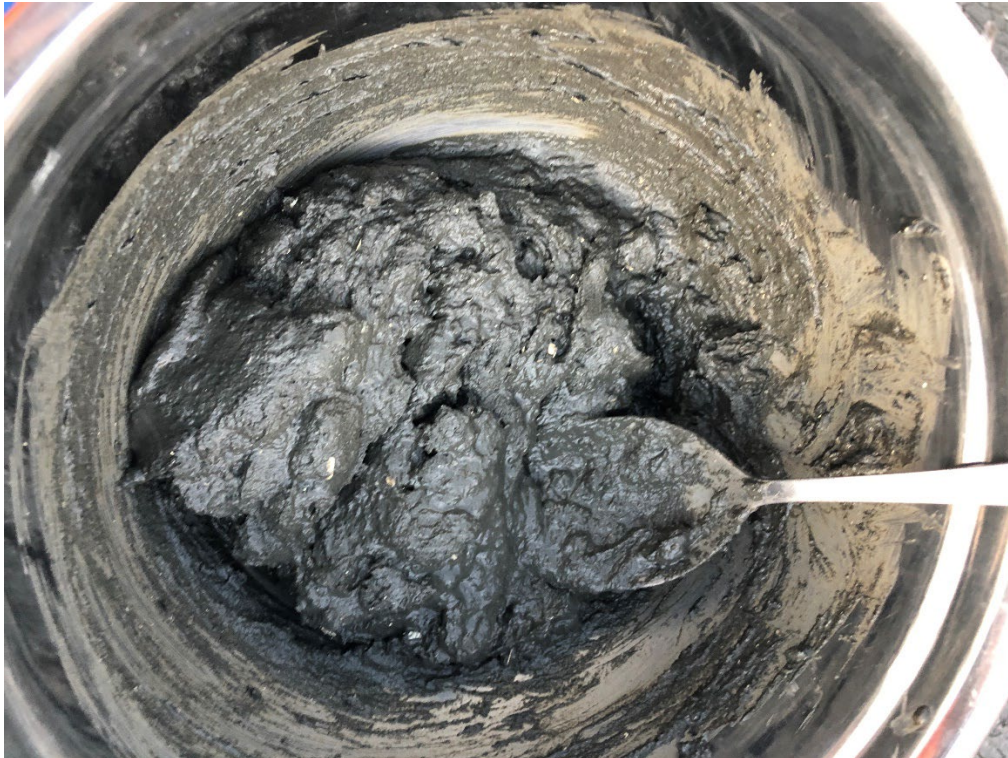
Photo #4: Homogenization and sampling of dredged material underway.
