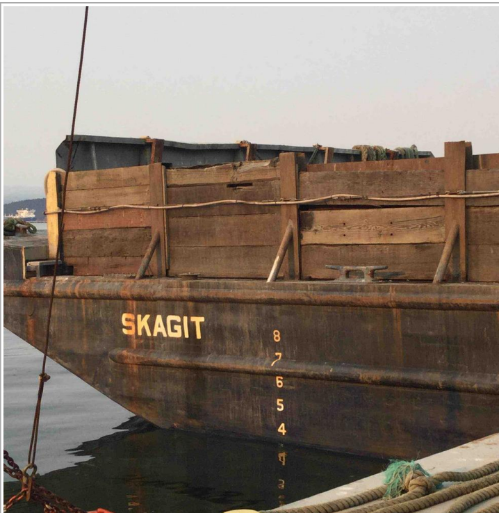
Barge draft at start of dredging.
