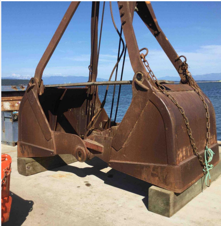
4 cubic yard rehandle bucket.
