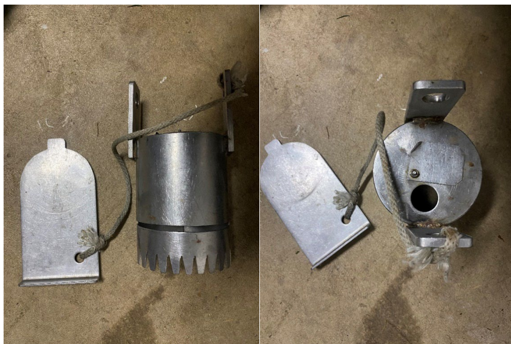
Figure 3 - Four-Inch Stainless Steel Hand Corer
