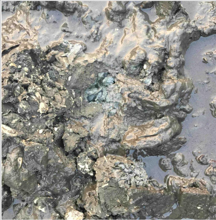
Patch of light grey silt/clay in grab for CPP3-W
