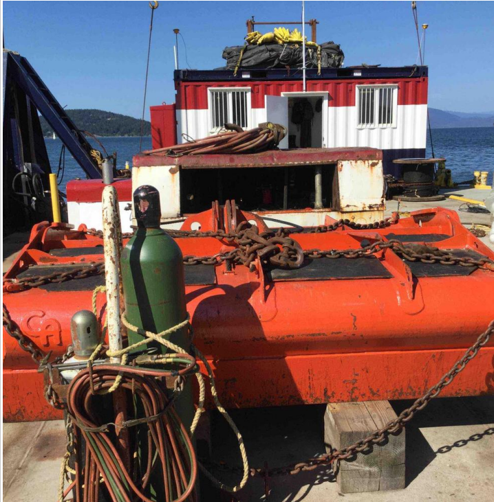
2 cubic yard cable arm (environmental bucket).
