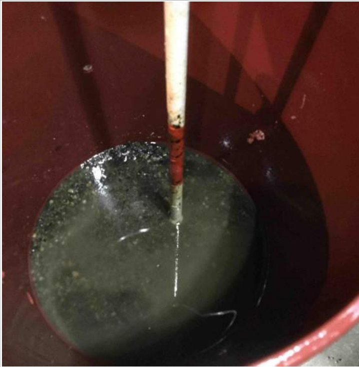
Rain bucket #24 measurements = 2" (pass)
