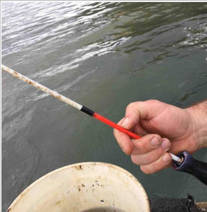
Rain bucket #6 within tolerance at 7 3/4"
