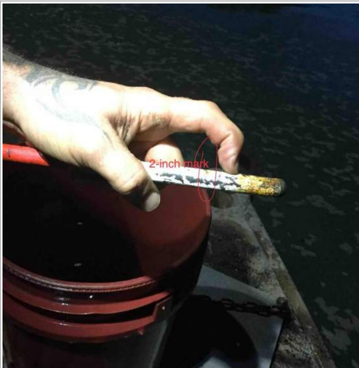
Rain bucket measurement, within 1-inch tolerance.
