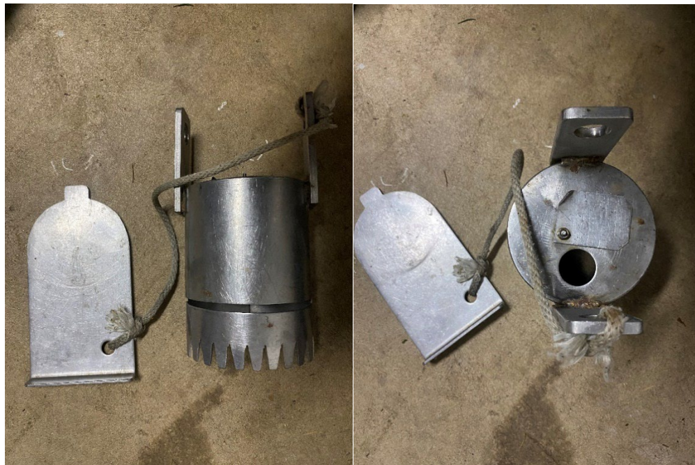
Figure 3. Four-Inch Stainless Steel Hand Corer
