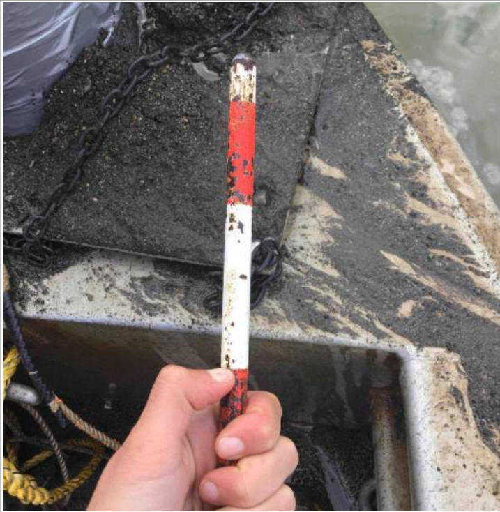
Rain bucket #28 measures at 6"(pass).
