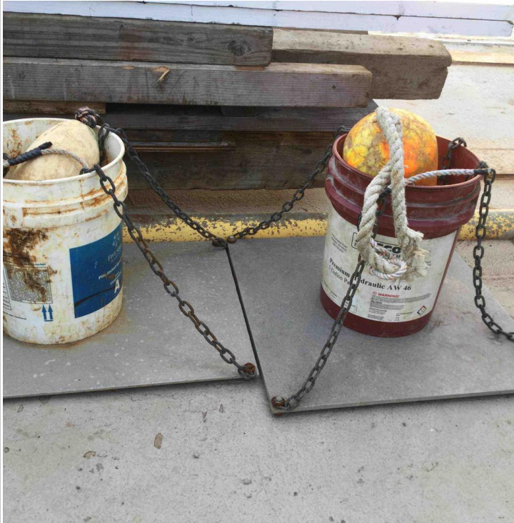
Rain buckets for verifying placement thickness (TLC)
