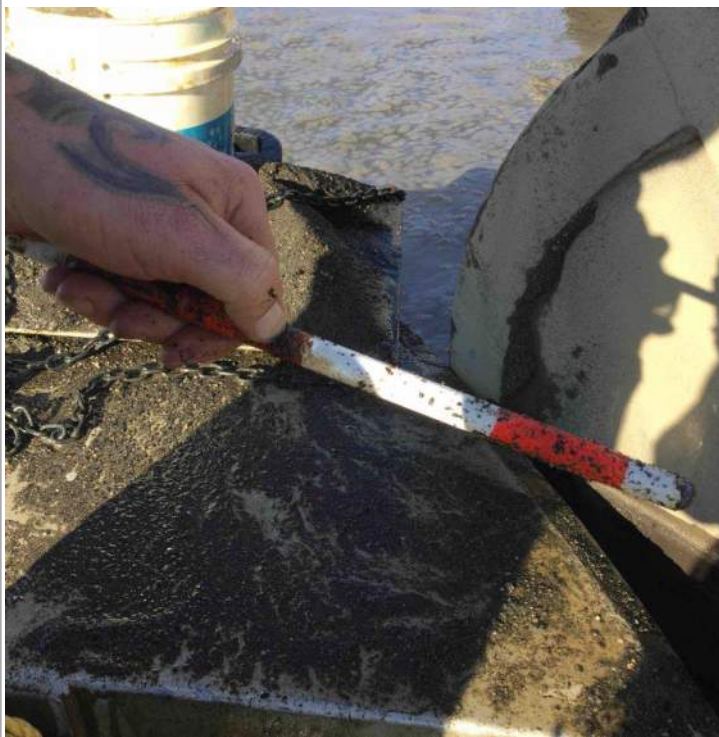
Measurement of RB #8 (6.5", 8.25" total)
