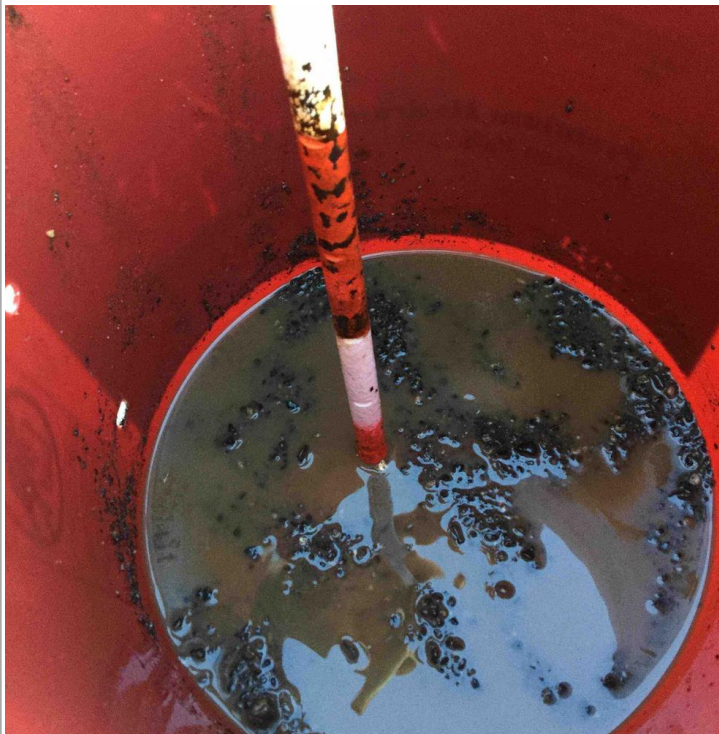
Rain bucket #33 measurement (1.75"= pass)
