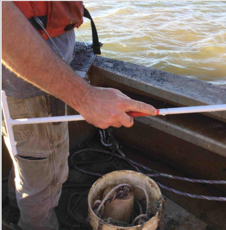
Depth of sediment on rod once removed from bucket (pointing at sediment level)
