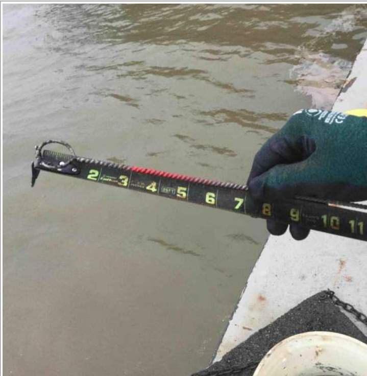
Rain bucket #22 measurement: 7" (pass)
