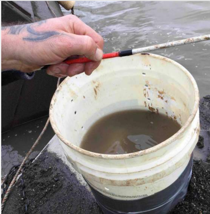
Rain bucket #12 measured within tolerance at 6 3/4"
