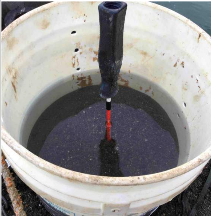
Rain bucket #15 measured within tolerance at 6 1/4".
