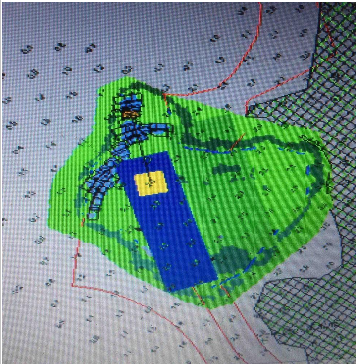
Bucket map for material placed in remaining low spots in dredge prism (blue ~ 6" low of threshold) (~13 x 4CY buckets placed)
