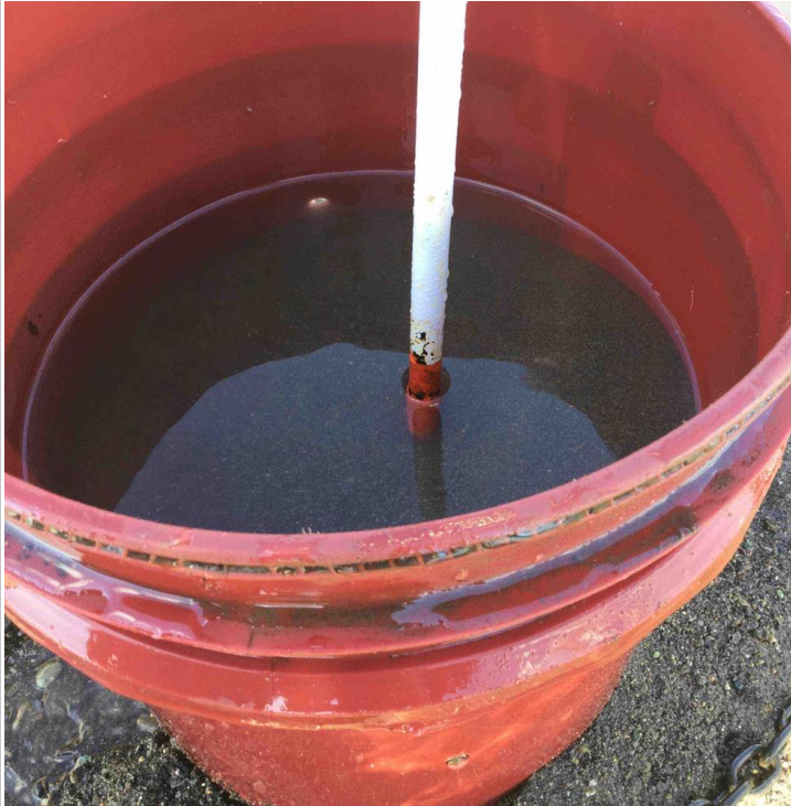
Rain bucket 4 measurement (8"= pass inspection)
