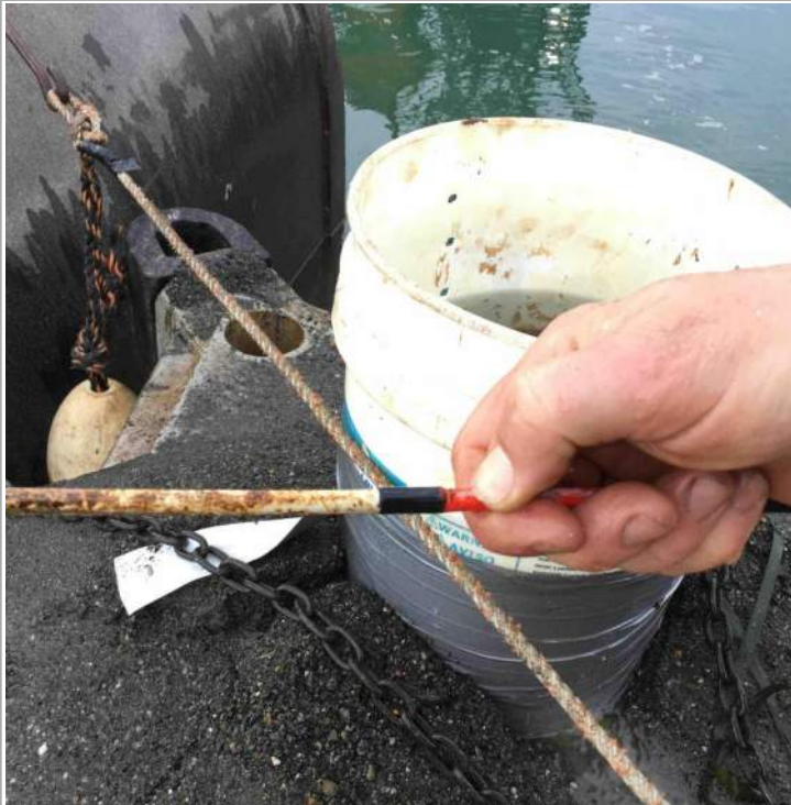
Rain bucket #1 measured within tolerance at 6 1/4".
