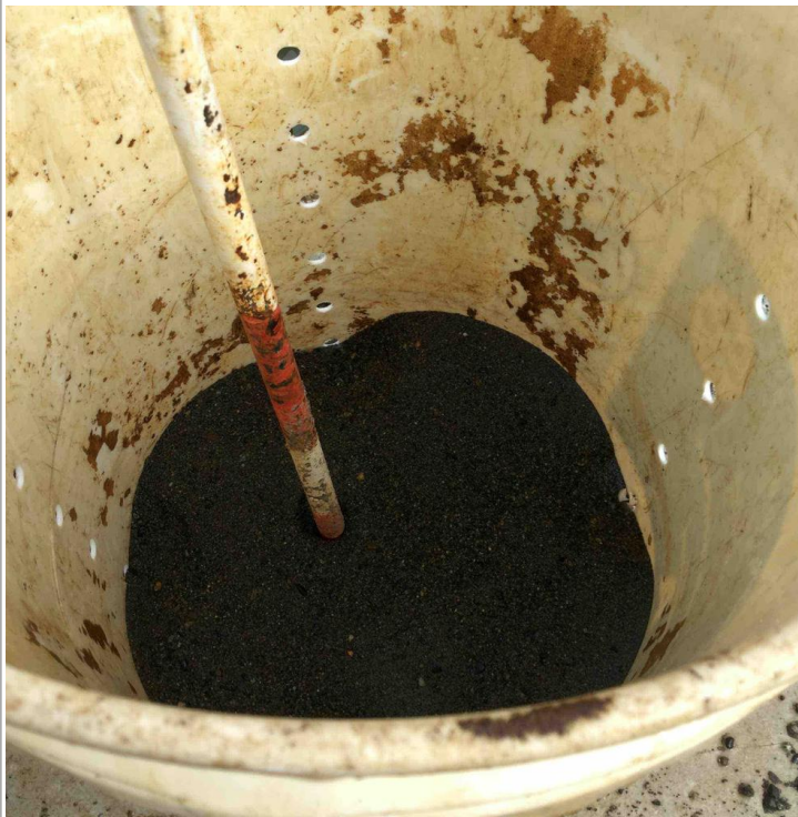
Measurement of rain bucket #30 (2"=pass)
