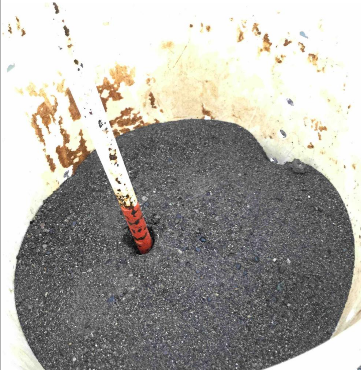
Measurement of rain bucket 4 = 8" (pass)
