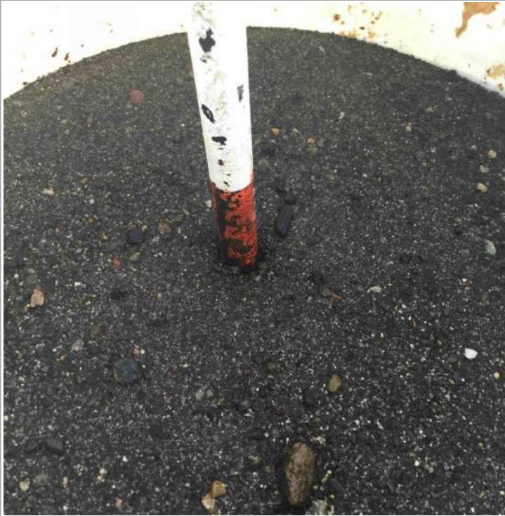
Rain bucket #13 measurement= 8" (pass)
