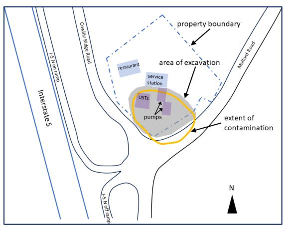
The property is located on the north side of the intersection of Mulford Road and Cowlitz Ridge Road. The area of soil excavation is shown in grey. The estimated extent of contamination is shown in orange. The existing underground storage tanks (USTs), fuel dispensers, and pumps will be removed before contaminated soil is excavated. If contaminated soil remains in the right of way under Mulford Road, then an environmental covenant will be filed with the county for the site. Areas are not exact.
