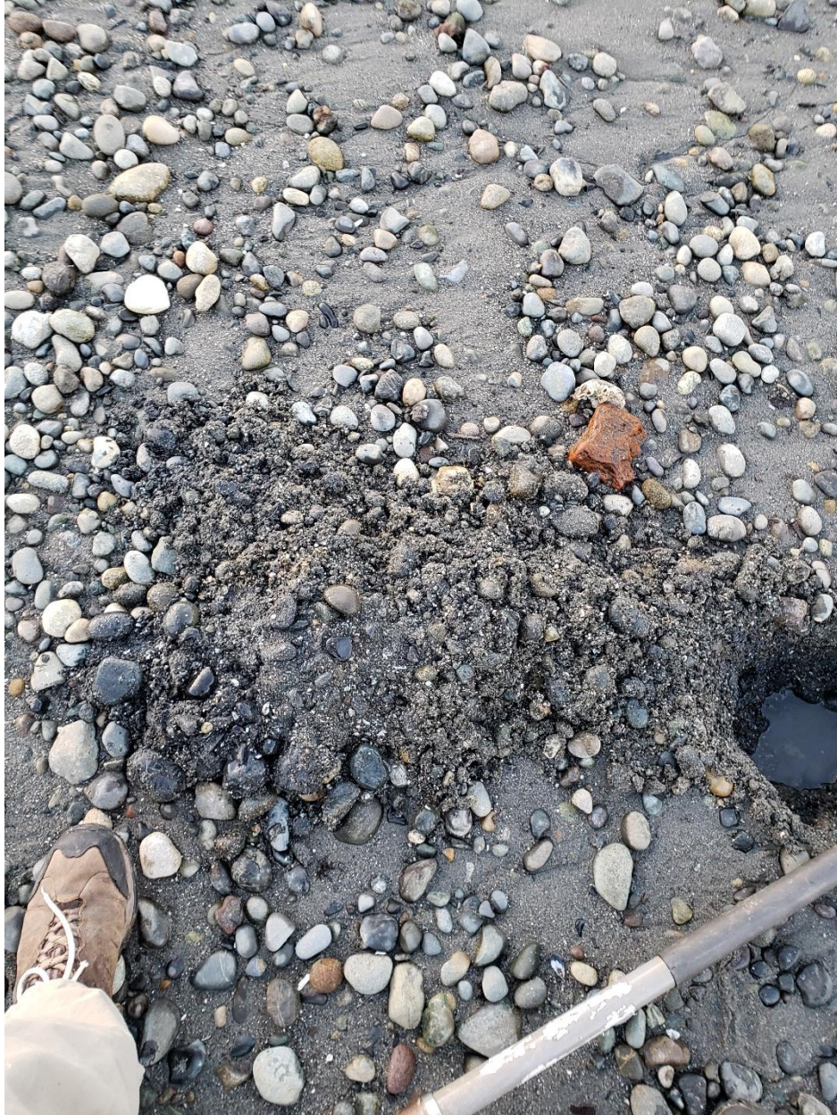
Figure 4. Cap Material Found in One of the Central Test Pits.
