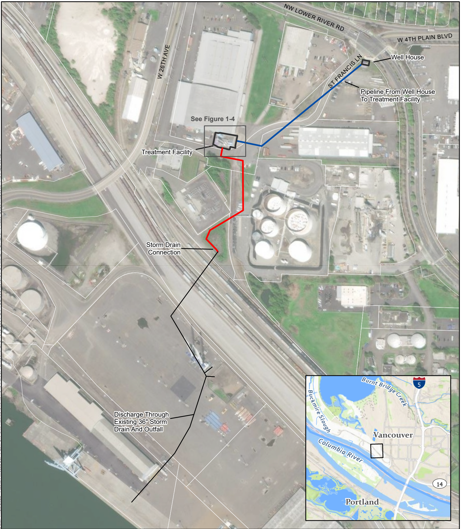
Figure 3 Groundwater Pump and Treat System Operation Plan - Cleanup Action Plan Groundwater Pump and Treat System Swan and Cadet Sites Port of Vancouver, WA
