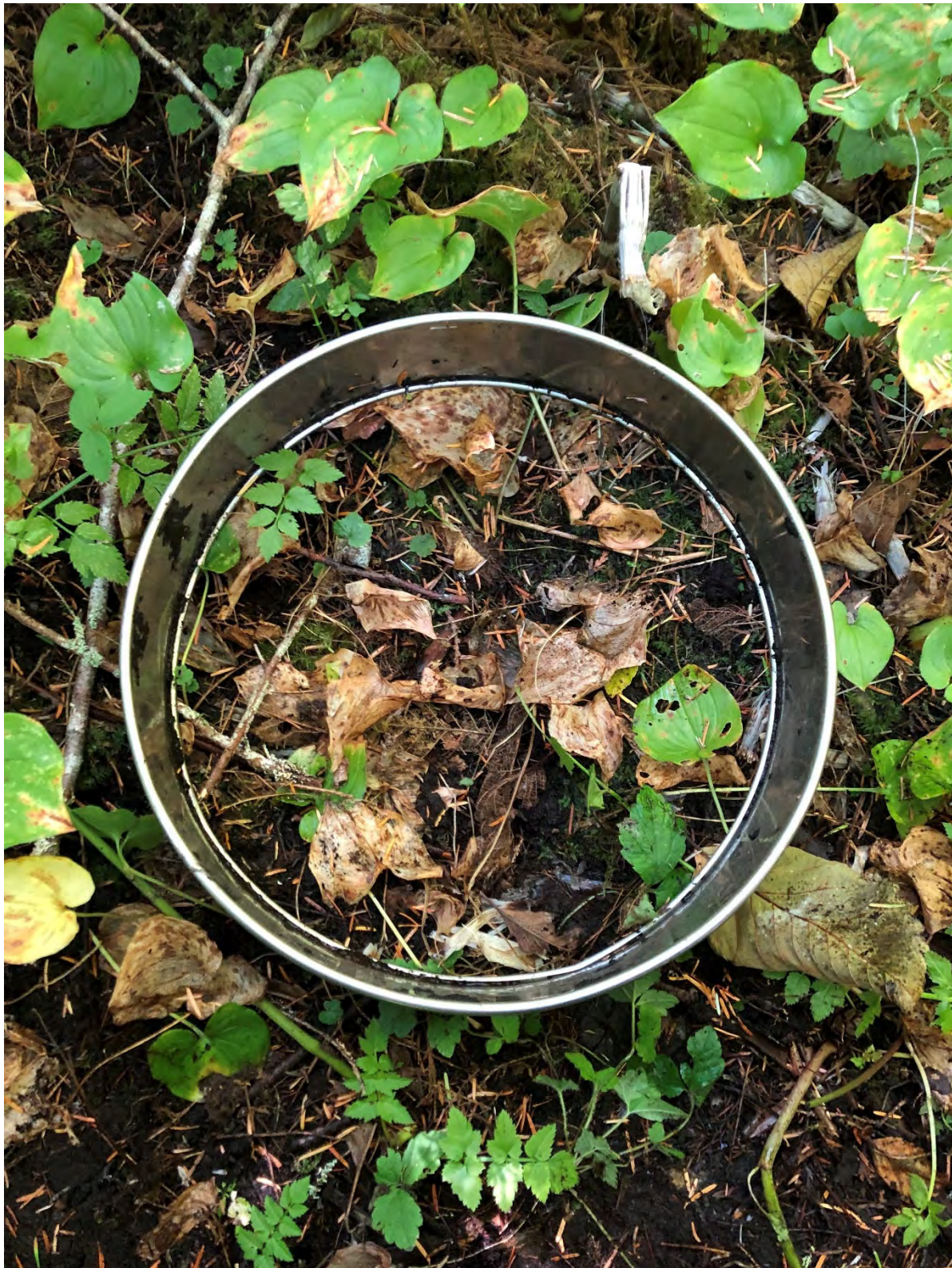
Photo 1: Initial placement of 12-inch diameter metal cylinder
