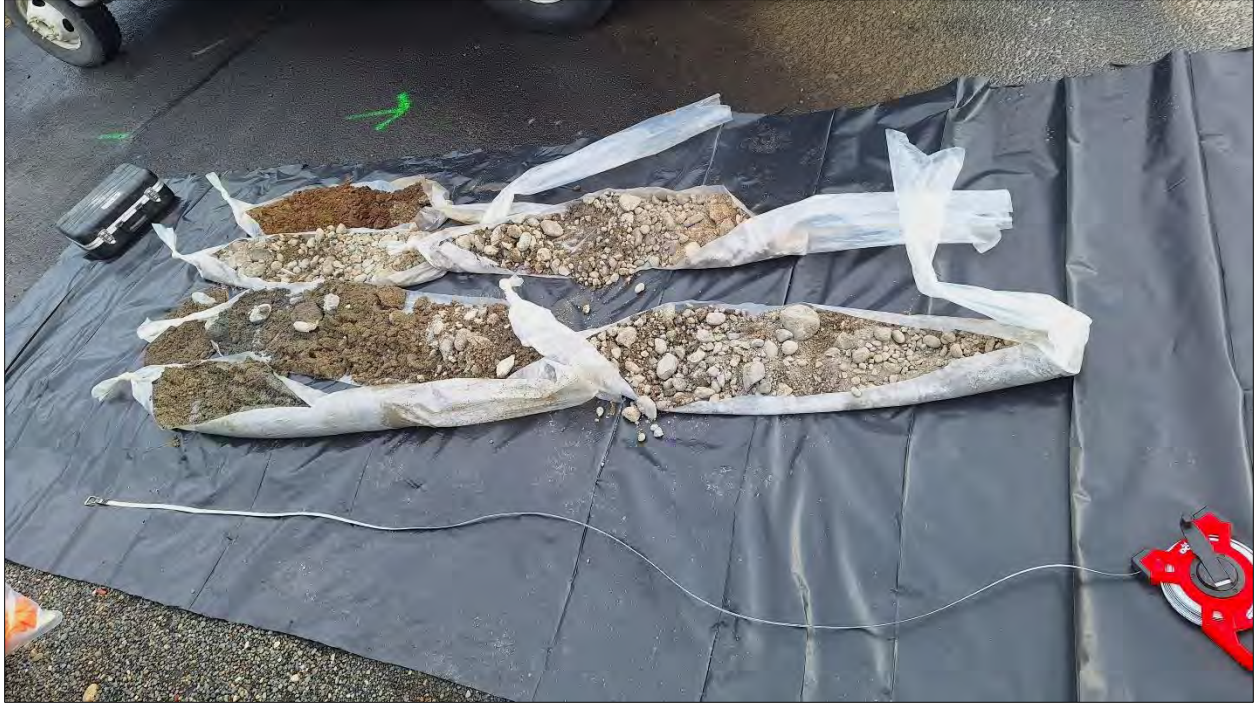
Figure 8. Oblique view of soil recovered from a borehole.
