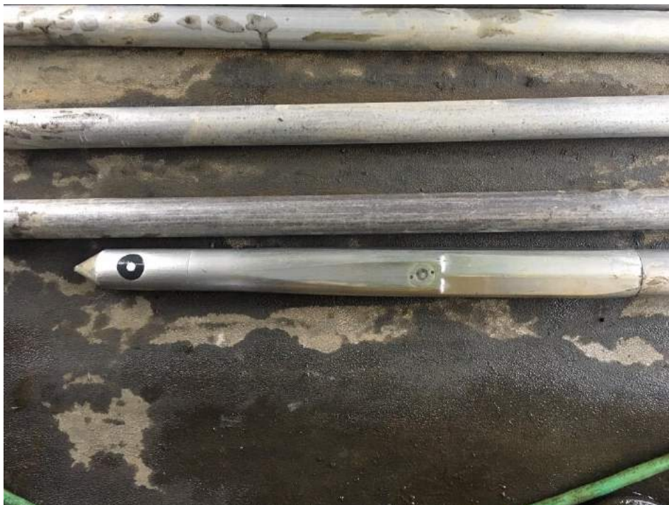
Photograph 2. OIP and HPT probe with rods.
