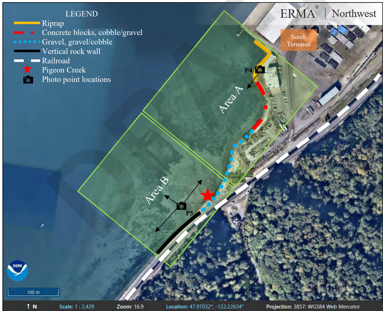
Figure 4. Southern shoreline conditions from the South terminal to the property boundary line south of Pigeon Creek (creek entrance onto shoreline noted by the red star). The shoreline is separated into two areas (A and B) represented by green boxes, and the legend describes the primary types of substrates present along the armored boundaries of the shoreline. Approximate Photo Point locations (e.g. “P4”) are indicated by the cameras, with arrows noting direction of photograph taken. Note that these locations are generalized, and roughly estimate what is present on Site.
