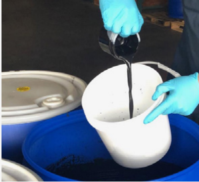
PetroFix is simply mixed with water and applied
