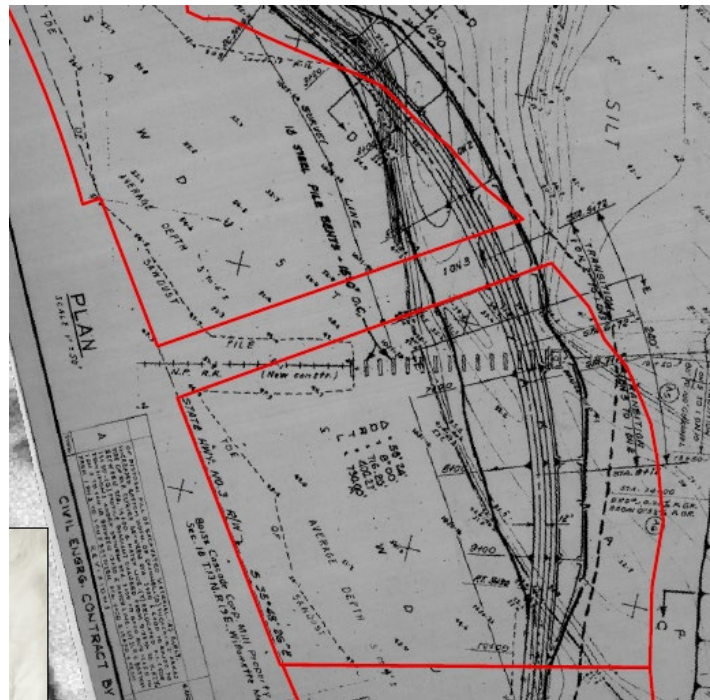
1966 Levee Repair Map with sawdust pile indicated on Parcels D & E (see Attachment C for the map)
