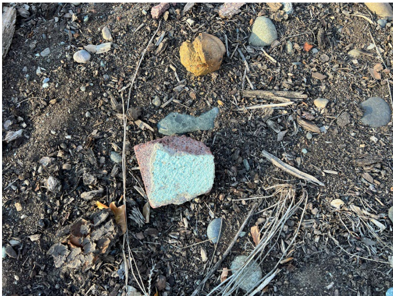
B11.3 Parcel D - A localized area of painted brick was present on the parcel.
