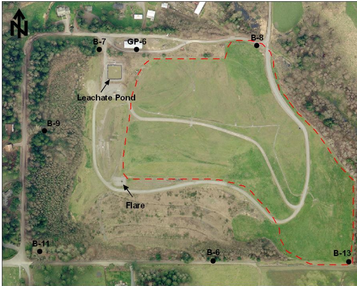
Figure 3. Perched Aquifer Monitoring Well Locations.
