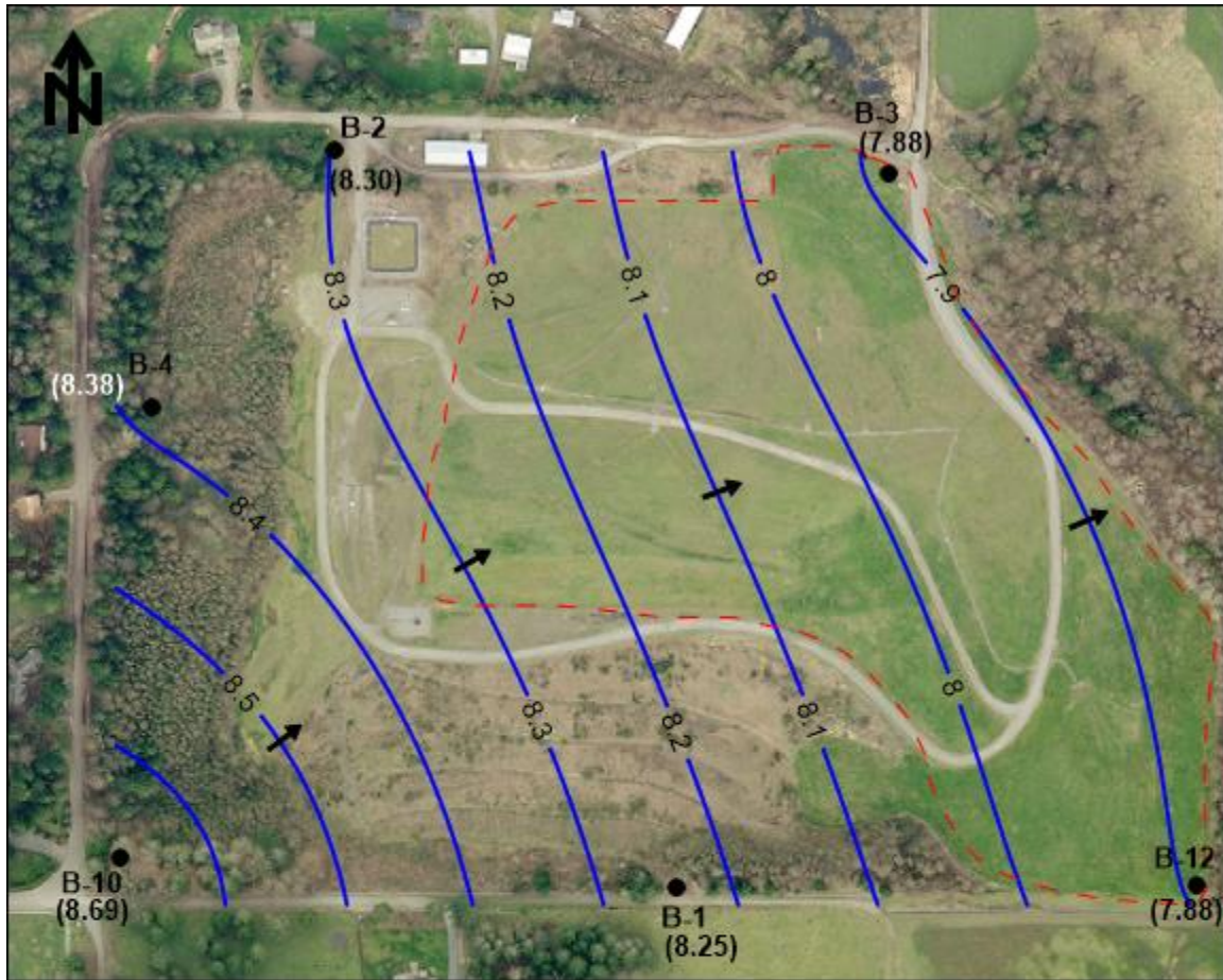
Figure 4c. Potentiometric Surface Contour, Central Landfill, Regional Aquifer, September 2023.
