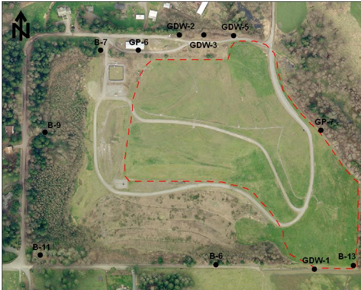
Figure 9. Landfill Gas Perimeter Monitoring Probe Locations.
