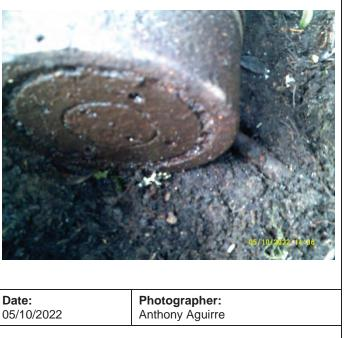
UXO 17 MEC: MK 38 mod 3 5" projectile APHE -Projectile base, tracer and bd fuze rings, Item ID: 1701
