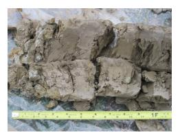
51.4 to 54.0' CLAY, some silt, medium to high plasticity; trace small to large pebbles, sub-round to sub-angular up to 2" diameter; moist, stiff, dark grayish brown (10 YR 4/2) NOTE: Lacustrine; laminated 0.1 to 0.2" thick, laminations brownish yellow (10 YR 4/3).
