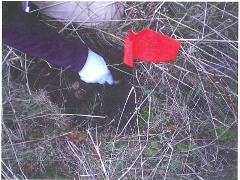
**USCG – Burrows Island Light Station:** *Photo 2* – View of soil being collected from a surface sampling location for laboratory confirmation analysis.
