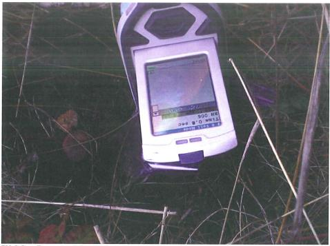
**USCG – Burrows Island Light Station:** *Photo 1* – View of X-ray Fluorescence (XL3t 600 Environmental Analyzer) equipment analyzing a soil sample through a Ziploc bag.
