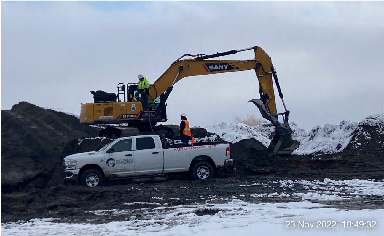
Photo 2: Pickup truck with fuel caddy refueling Sany 215C LC trackhoe.
