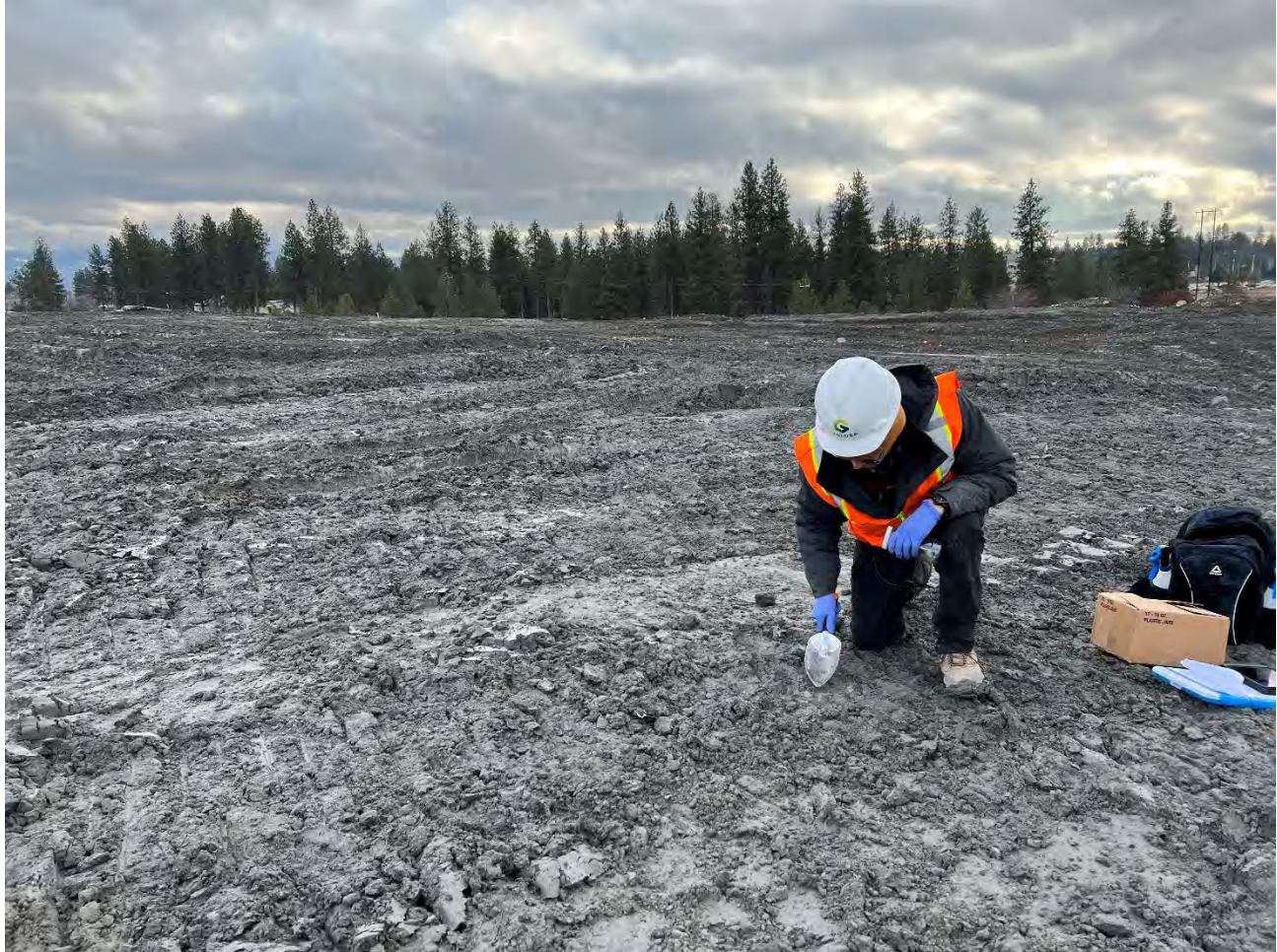
Photograph 2: Collection of confirmation sample for UPRR-2 at randomly selected grid centroid.
