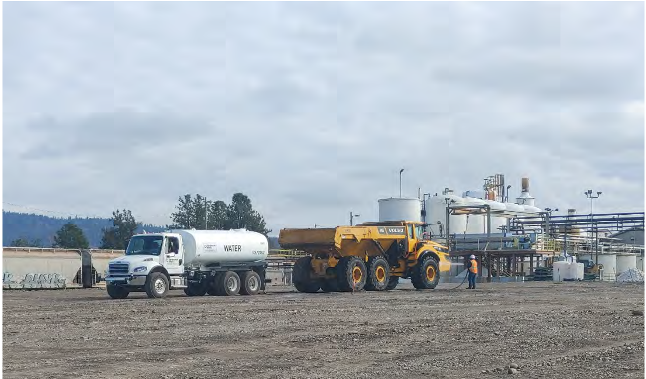
Photograph 4: Cleaning the Volvo A45G Off-Road Haul Truck using the water truck and a power washer to be sent offsite later today (4/13/2023).
