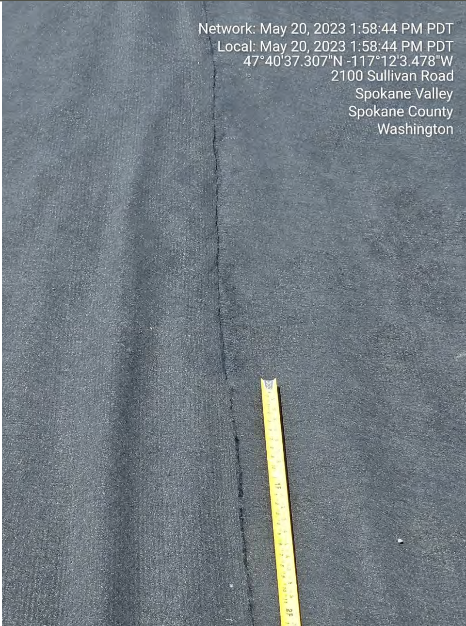
Photograph 5: Typical seam weld at top of picture and transition to unwelded portion of the seam bottom adjacent to the tape measure.
