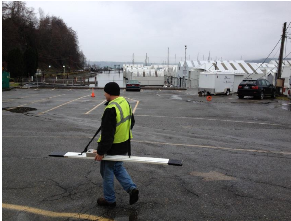
Figure 3. The Geophex GEM-2 Electromagnetic Instrument collecting data at a UST Site in Tacoma, WA.
