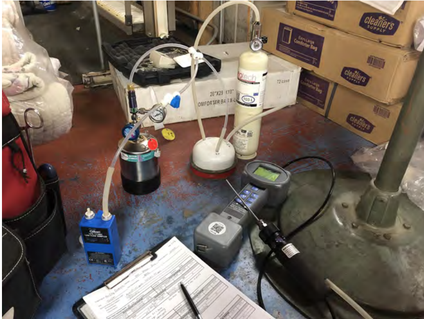
Photograph 9. Sub-slab soil vapor sampling train and equipment. This example photo was taken at VP-06.
