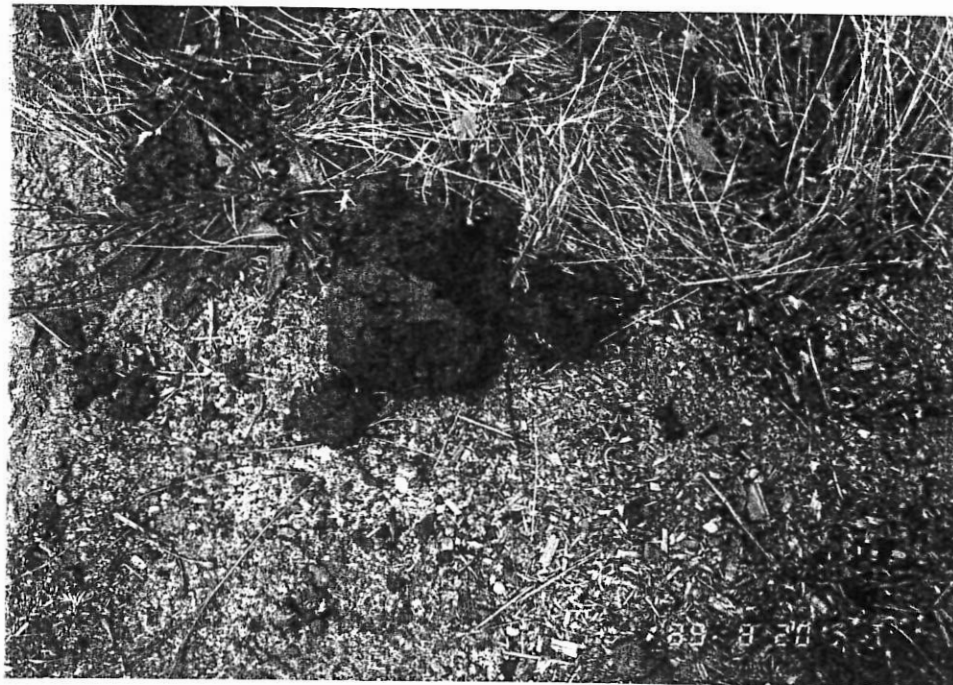
PHOTO NO. 4. Close up view of petroleum-contaminated clayey wetland soil collected from below the sandy dredge material under UST no. 10. This soil was discolored dark grayish blue and had a moderate diesel odor.
