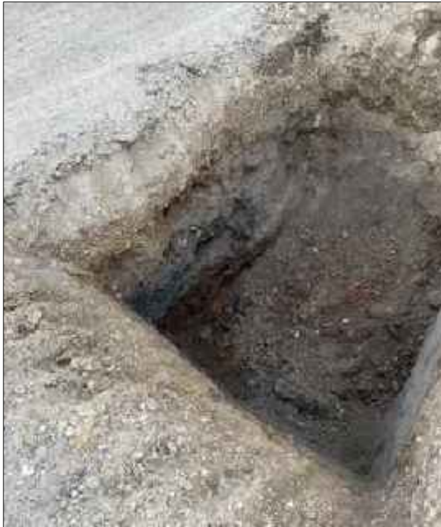
PHOTO 4 Abundant bark and wood debris at 5' bgs in Excavation 2.
