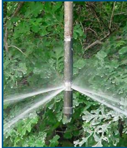
FIGURE 6 Image of Geoprobe ® pressure activated injection probe
