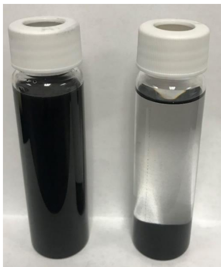
Figure 1- Two vials containing 2,000 mg/L of CAC. The recommended dose of settling agent was also added to the vial on the right, resulting in clear water.
