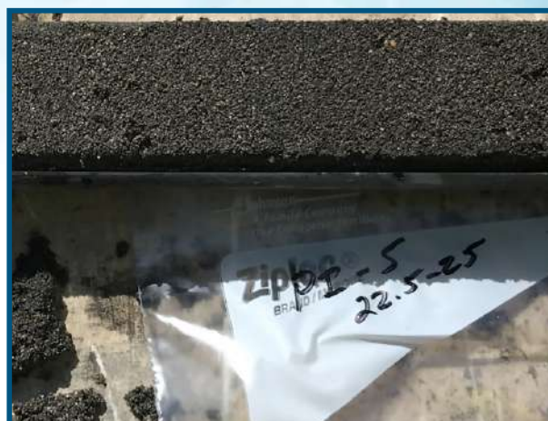
FIGURE 1 The photo on the left shows a soil core collected before a PetroFix application. The photo on the right shows a soil core collected after a PetroFix application exhibiting black soil where the PetroFix was successfully distributed.
