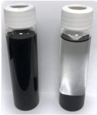
Figure 1 – Two vials containing 2,000 mg/L of CAC. The recommended dose of settling agent was also added to the vial on the right, resulting in clear water.
