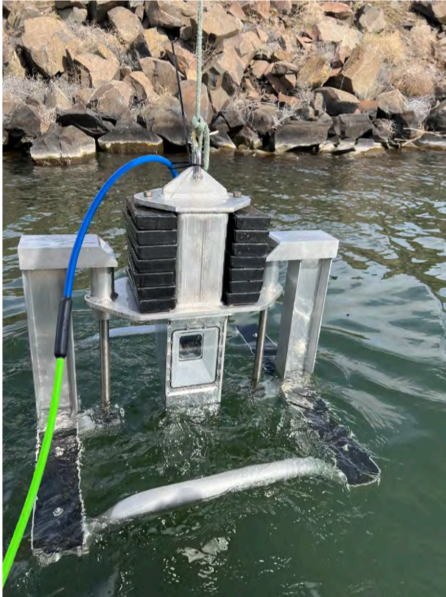
Figure 2 Sediment Profile Imagery (SPI) System
