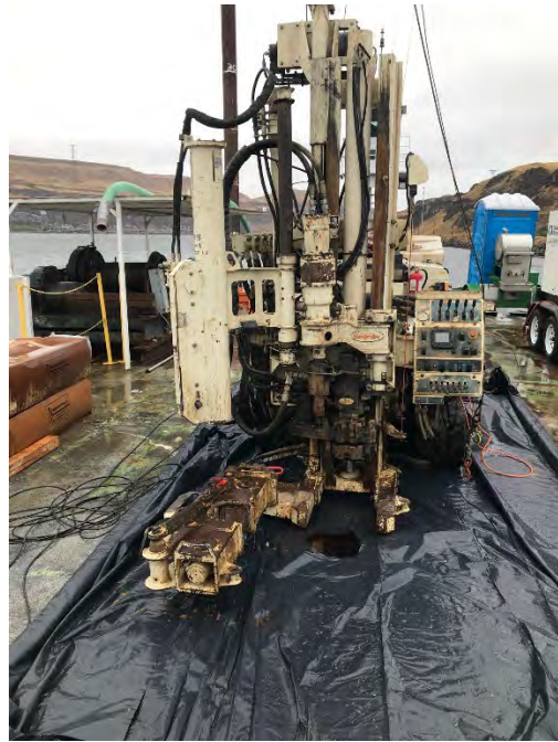
Photograph 6: Drill Rig Set Up for Core Collection Date taken: 11/01/2022
