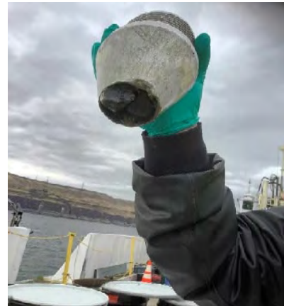
Photograph 42: K360 Attempt 2 Material stuck in drill shoe
