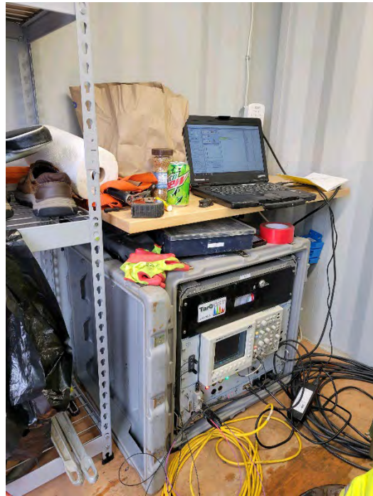
Photograph 4: TarGOST Equipment Set Up Date taken: 11/01/2022
