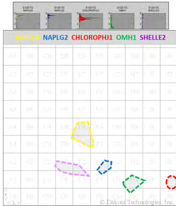
Figure 11. Cluster diagram overlay of the Basis Set waveforms used in the NNLS processing employing dashed lines with colors that match the NNLS Basis set waveform colors.
