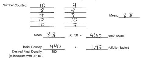
Prepare the embryo inoculum according to the calculated dilution factor. For example, if the dilution factor is 2.25, use 100 ml of existing stock (1 part) and 125 ml of dilution water (1.25 parts).
