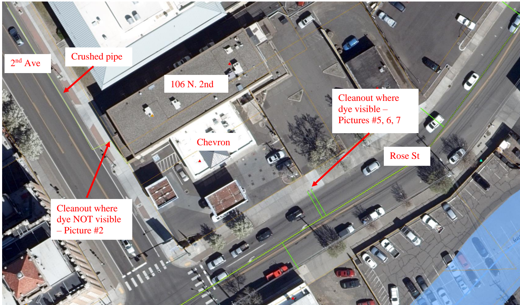
Figure 1: Map of area where dye testing performed and location of known sewer lines (Source: City's GIS mapping)
